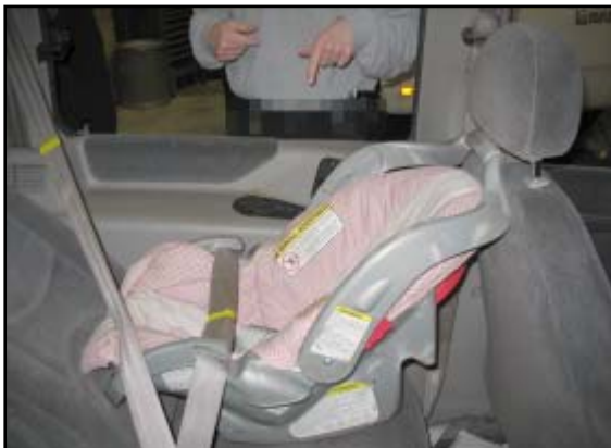
Figure 11. Reinstalled RFCSS using the belt path.
