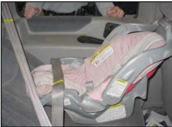
Figure 14. RFCSS with the lap positioned across the rear of the safety seat.
