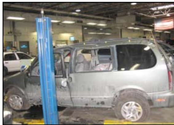
Figure 5. Left side damage and roof side rail crush profile.
