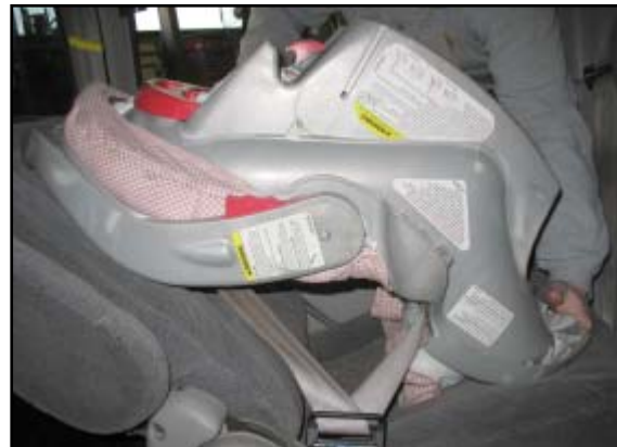
Figure 12. Front-to-rear rotation of the safety seat. The webbing remained engaged with the belt path during this simulation.
