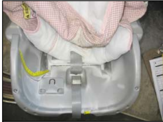
Figure 16. Stress marks and fracture at the right belt path.
