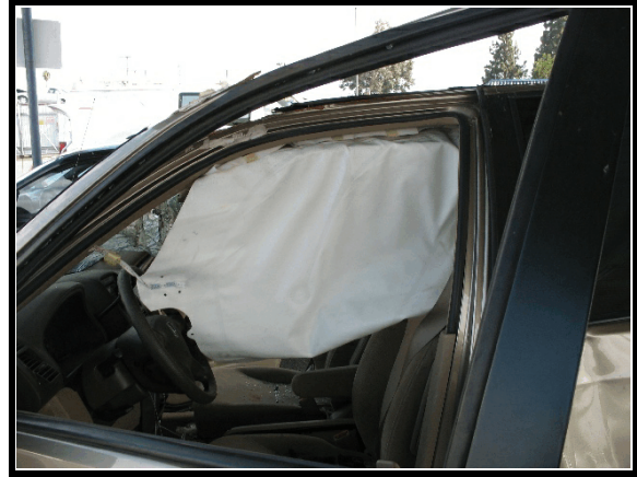
Figure 14. Left side air curtain. Outside view at driver's location.
