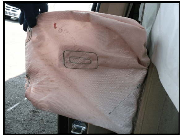
Figure 10. Front right passenger side air bag
