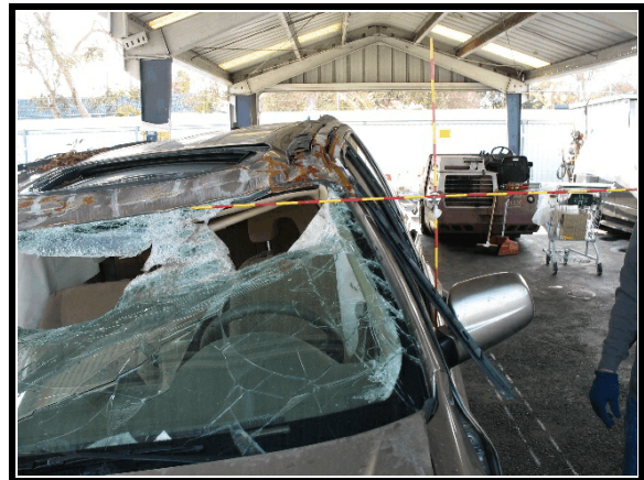
Figure 8. Maximum vertical crush
