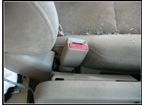
Figure 9. Driver's compressed seat belt latch
