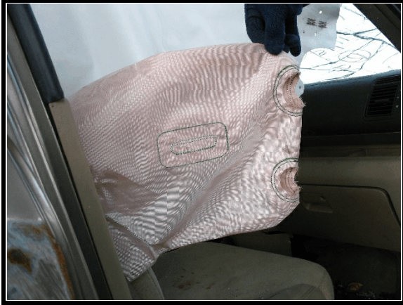
Figure 11. Front right side air bag (exterior view)
