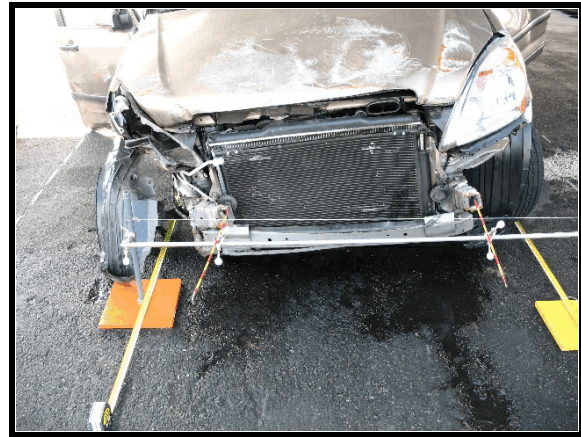
Figure 4. Front end damage, Honda CR-V
