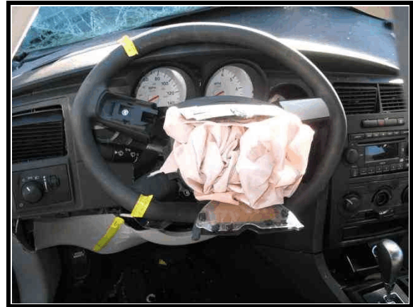
Figure 9. Steering wheel rim loading
