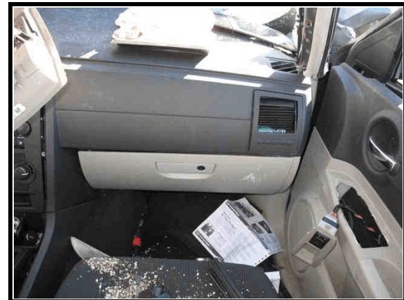
Figure 8. Deployed front right passenger air bag
