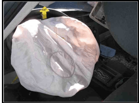
Figure 7. Deployed driver's air bag
