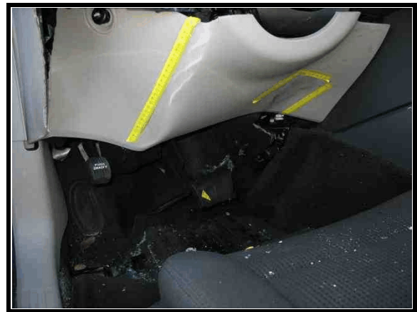
Figure 6. View of lower instrument panel contacts/damage
