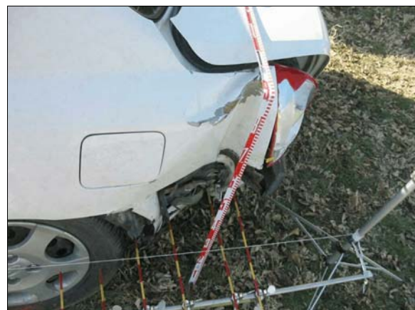
Figure 11: Left quarter panel damage from sign impact, vertical scale in tenths of meter, each increment on rods is 5 cm (2 in)
