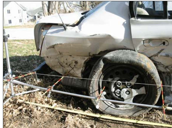
Figure 10 Damage to right rear wheel, right rear door and quarter panel
