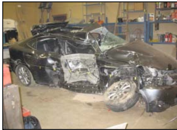
Figure 6. Resultant right side damage from the impact with the Ford.
