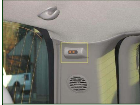
Figure 7. URPA display on the right D-pillar.
