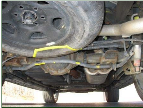
Figure 14. Undercarriage contact evidence to the spare tire and rear sway bar.
