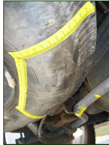
Figure 15. Right lateral view of the spare tire wipe mark.
