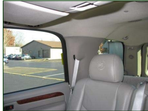
Figure 17. Additional view of the C-pillar blind spot.
