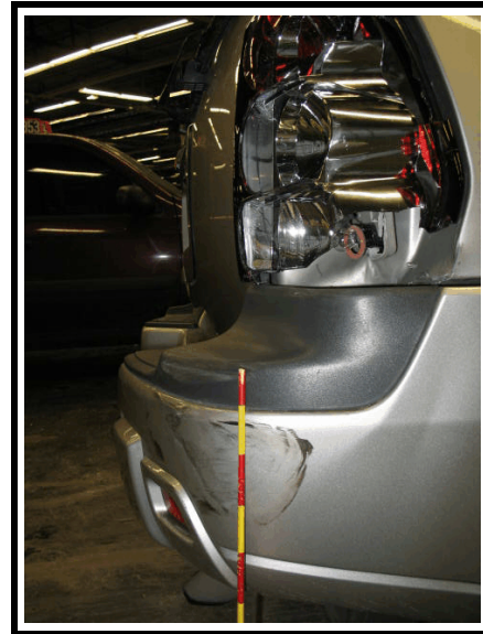
Figure 12. Right rear bumper corner/taillight damage
