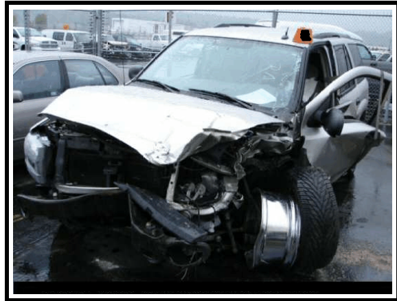
Figure 7. Debeaded LF tire (not with vehicle at the inspection)
