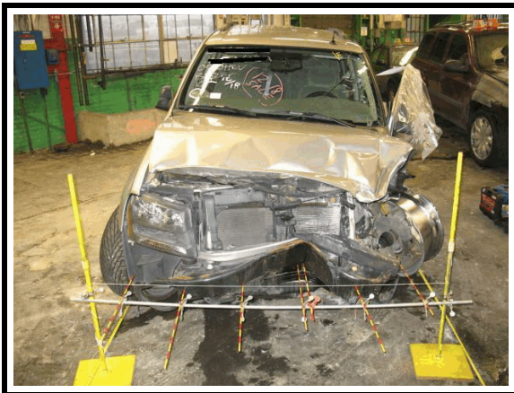
Figure 8. Front crush profile - bumper level
