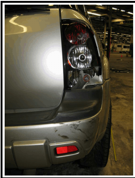
Figure 11. Back/right damage from secondary impact
