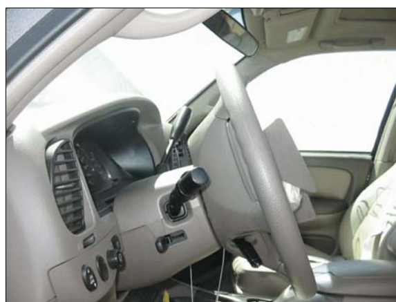
Figure 5: Left side view of case vehicle's steering wheel and steering column showing lack of deformation
