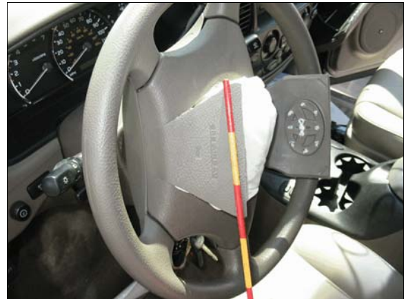
Figure 6: Case vehicle's driver air bag cover flaps, each stripe on rod is 5 cm (2 in)
