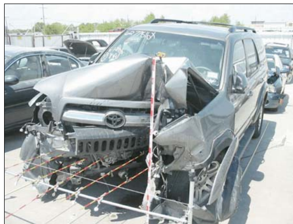
Figure 2: Overview of damage to front of case vehicle from impact with luminaire pole
