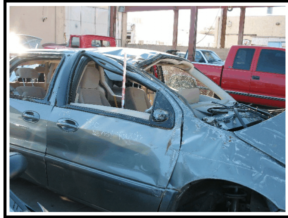
Figure 12. Right side passenger compartment rollover damage
