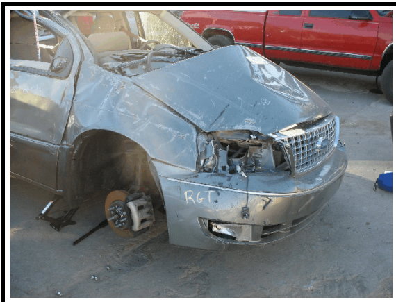
Figure 13. Right front rollover damage (RF tire removed/sold by wrecking yard)
