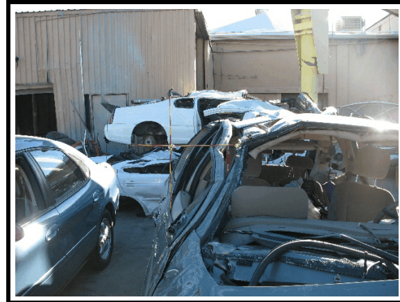
Figure 14. Location of max crush from the rollover event (right A pillar)
