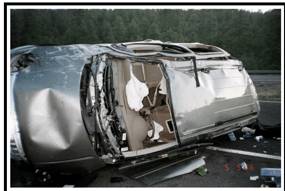
Figure 10. Windshield damage at the scene (police photo)
