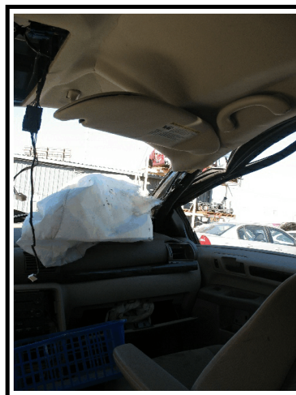
Figure 31. RF passenger's seating area & displaced roof-mounted light
