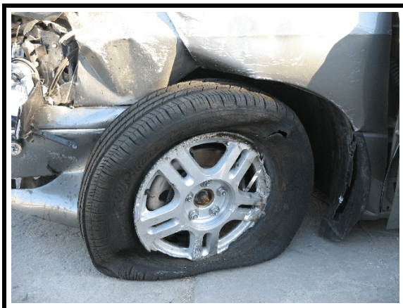
Figure 7. Left front tire/rim damage
