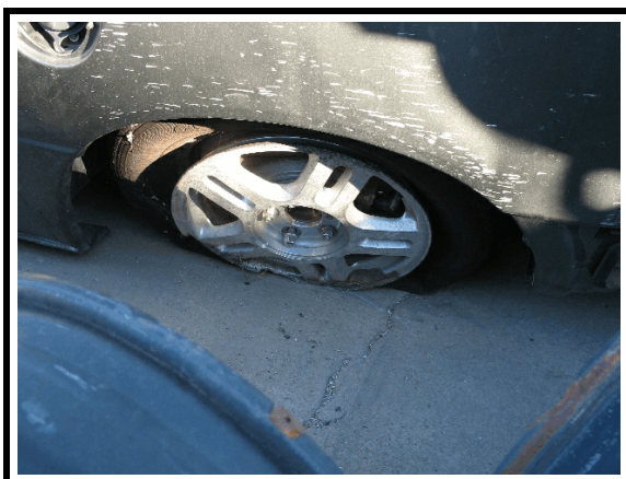
Figure 8. Left rear tire/rim damage
