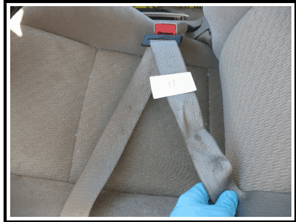
Figure 29. Evidence of occupant loading to driver's seat belt
