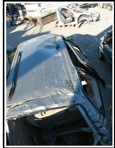
Figure 9. Rollover damage & opening at upper right rear door
