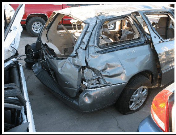
Figure 11. Right rear rollover damage
