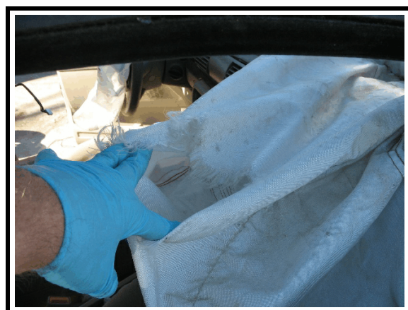
Figure 27. Damage to deployed passenger front air bag
