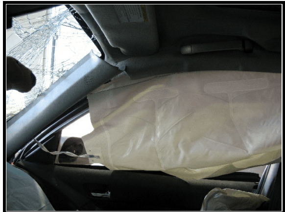
Figure 12. Right side air curtain at A pillar
