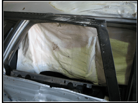
Figure 10. Overview of side curtain at right rear location
