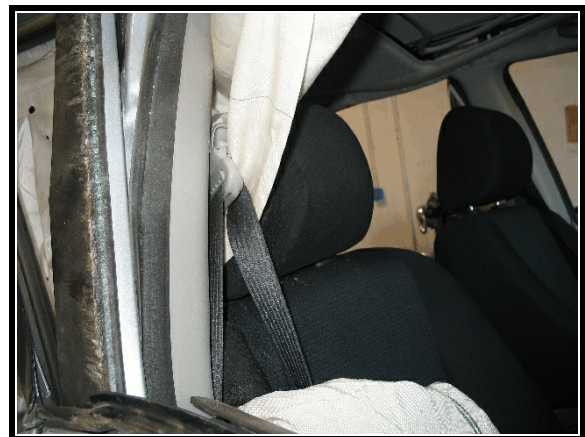
Figure 14. Side air curtain entrapped by head restraint at B pillar
