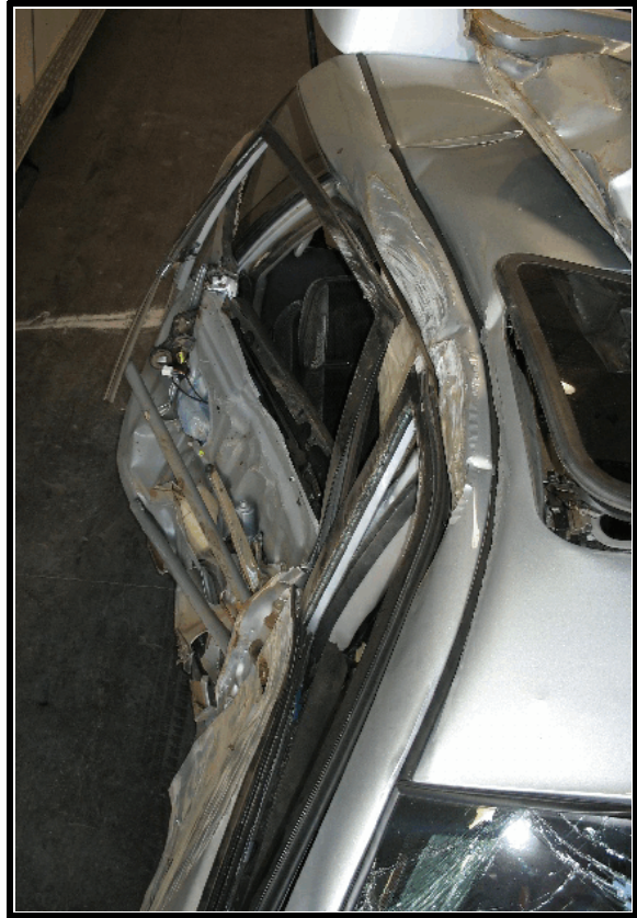
Figure 5. Overhead view of right side crush
