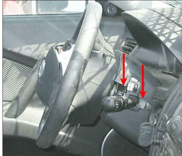
Figure 8: Case vehicle's energy absorbing steering column was compressed separating the steering column cover at assembly seam (arrows)
