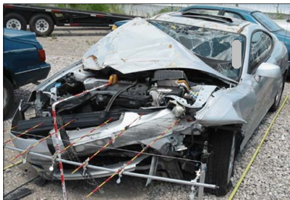
Figure 2: Damage to front of case vehicle from concrete median barrier impact and to top plane from rollover, increments on vertical scale are in tenths of meter, each increment on rods is 5 cm (2 in)
