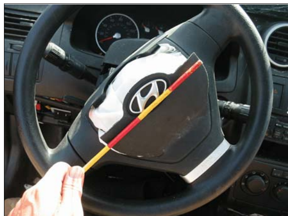
Figure 9: Case vehicle driver's air bag module cover flaps
