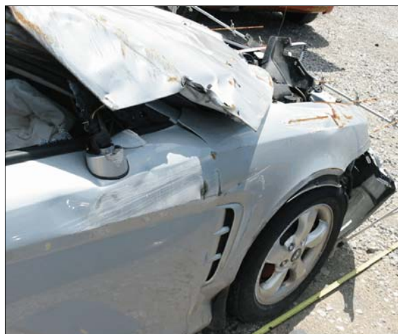
Figure 4: Rollover damage to right fender, hood, and right front door
