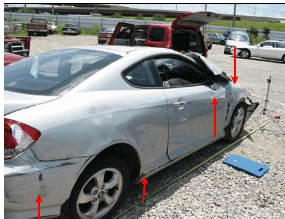
Figure 3: Overview of rollover damage (arrows) to right side of case vehicle
