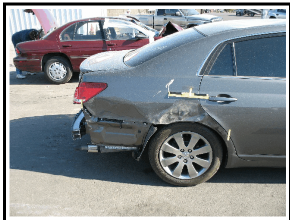
Figure 2. Right rear damage - 2005 Toyota Avalon
