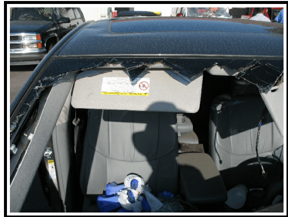
Figure 15. Windshield damage - right side
