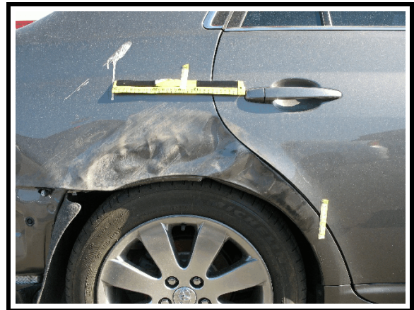
Figure 10. Beginning of right rear damage
