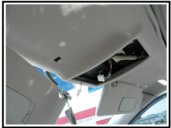
Figure 17. Roof mounted light and rearview mirror displaced
