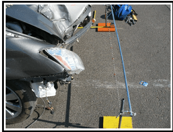
Figure 12. Front crush profile
