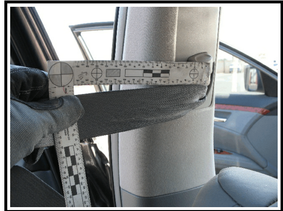
Figure 20. Evidence of loading to driver's seat belt
