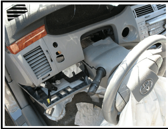
Figure 18. Instrument panel damage/intrusion & shear module separation
