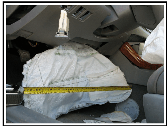
Figure 22. Deployed driver's knee air bag
