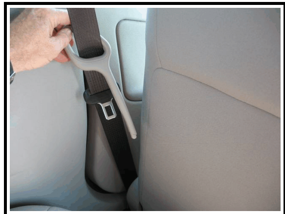
Figure 8. Broken left front seat belt positioning device (belt not in use at time of crash)
