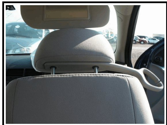
Figure 9. Intact right front seat belt positioning device (for comparison)
