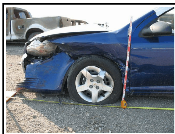
Figure 6. Left front damage - 2006 Chevrolet Cobalt
