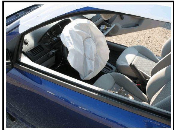
Figure 10. Deployed driver's front air bag
