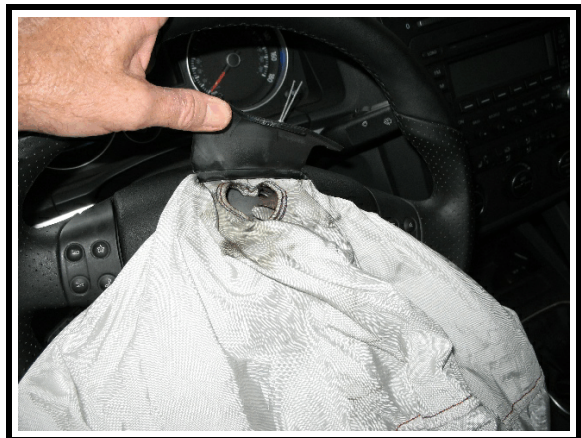
Figure 9. Driver’s front air bag vent port
