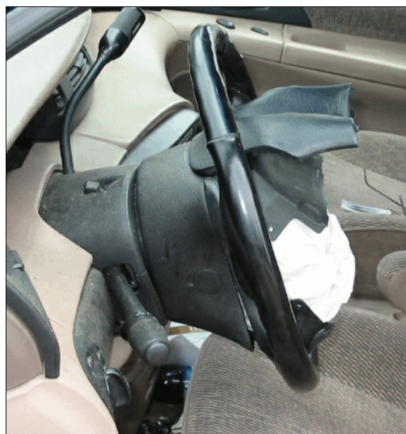
Figure 10: Left side view of case vehicle’s steering wheel showing lack of deformation
