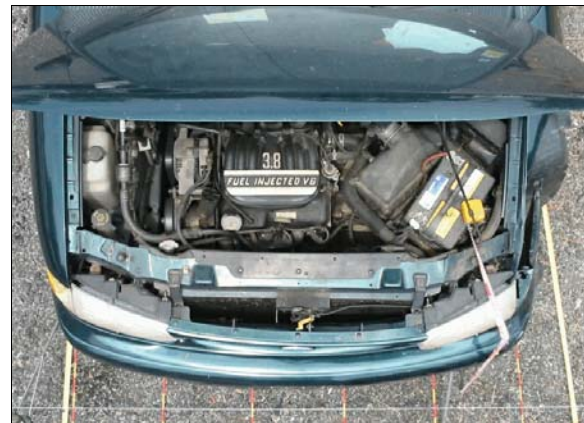
Figure 8: Top view of crush to case vehicle’s front bumper [baseline placement subsequently reduced 10 centimeters (4 inches) to establish case vehicle’s specification overall length, each increment on rods is 5 cm (2 in)]
