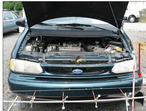
Figure 3: Overview front of case vehicle, arrow shows direct damage to front left bumper corner due to impact with tree
