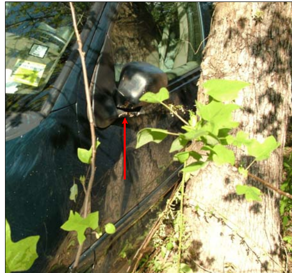
Figure 6: Arrow shows displacement of left side view mirror and bark transfer on mirror due to impact with the tree
