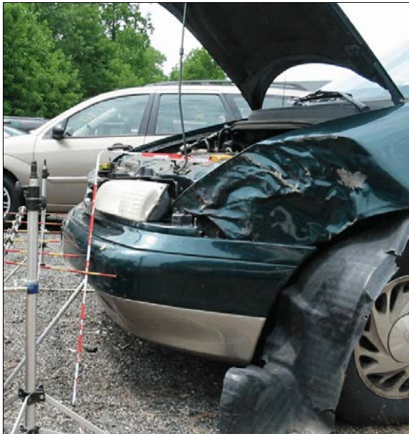
Figure 5: Damage to left corner of front bumper and left fender due to impact with the tree
