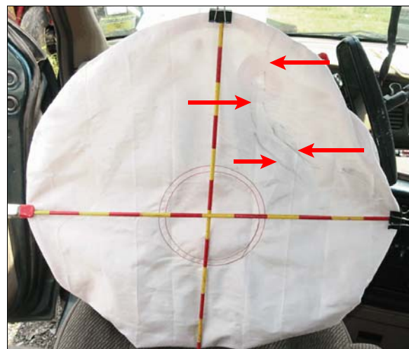
Figure 13: Case vehicle's driver air bag, arrows shows semi-circular black scuffs on air bag
