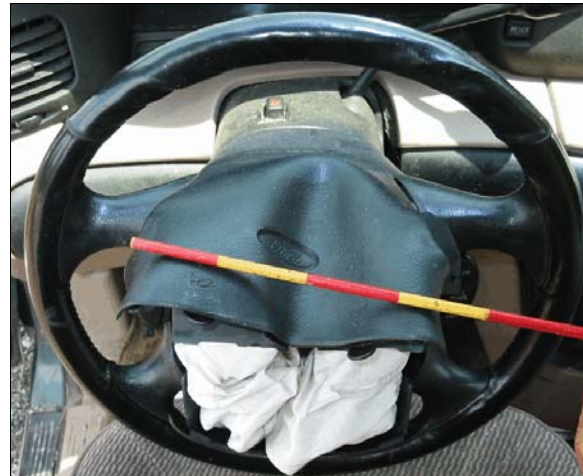
Figure 11: Deformation to top cover flap due to interaction with front left occupant during air bag deployment
