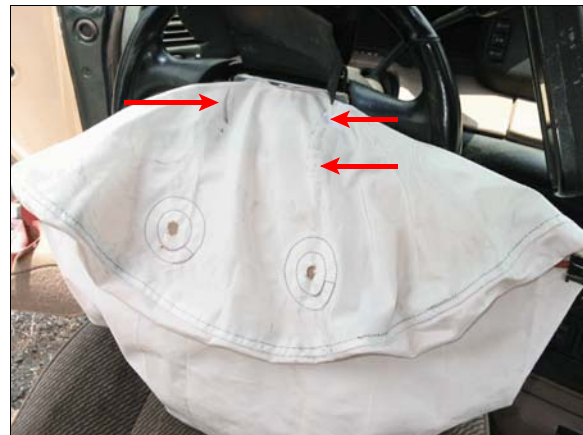
Figure 12: Arrows show linear black scuff marks on back of driver's air bag due to contact with back of top cover flap
