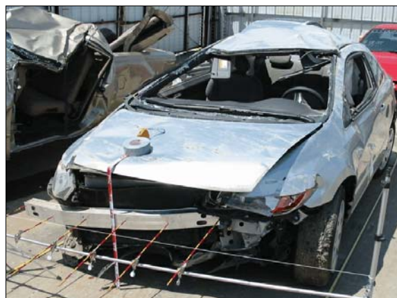
Figure 2: Overview of damage to front of case vehicle from impact with median barrier and damage from roll over, increments on tape measure on hood are in tenths of meter, each increment on rods is 5 cm (2 in)
