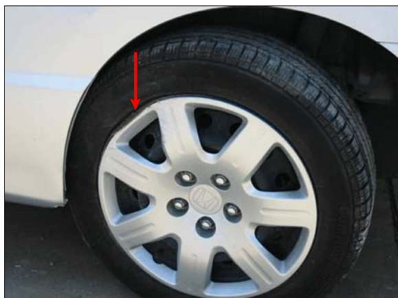
Figure 3: Damage to left rear wheel (arrow) from impact with median barrier, wheel angled in at bottom
