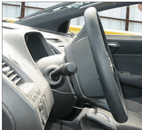
Figure 12: Left side view of case vehicle's steering wheel and steering assembly showing lack of deformation
