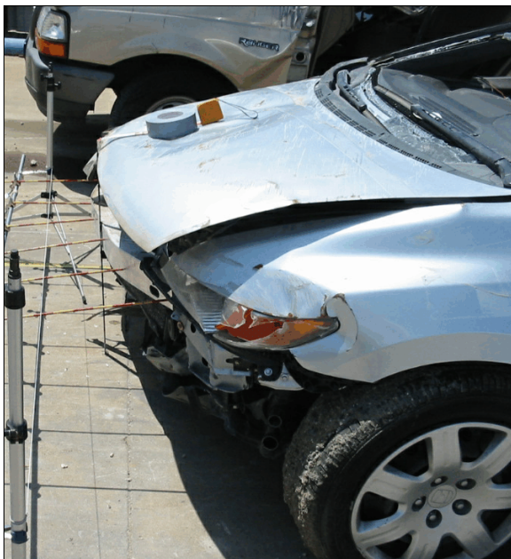
Figure 7: Left side view of crush to front of case vehicle
