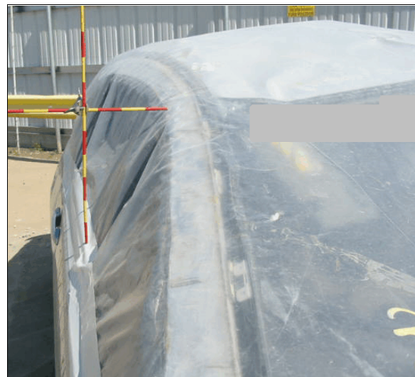
Figure 9: Case vehicle’s maximum lateral crush located at top of right “A”-pillar
