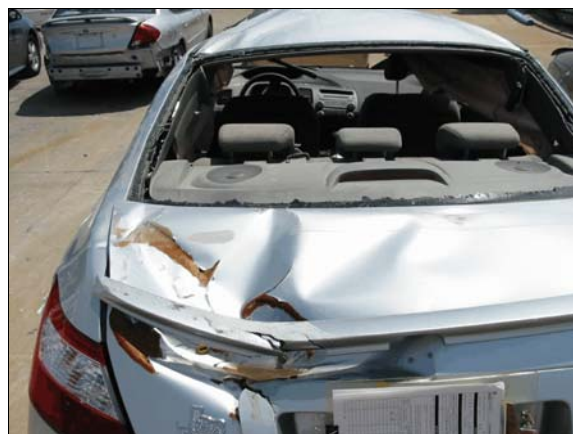
Figure 4: Damage to trunk lid from impact with top of median barrier during rollover
