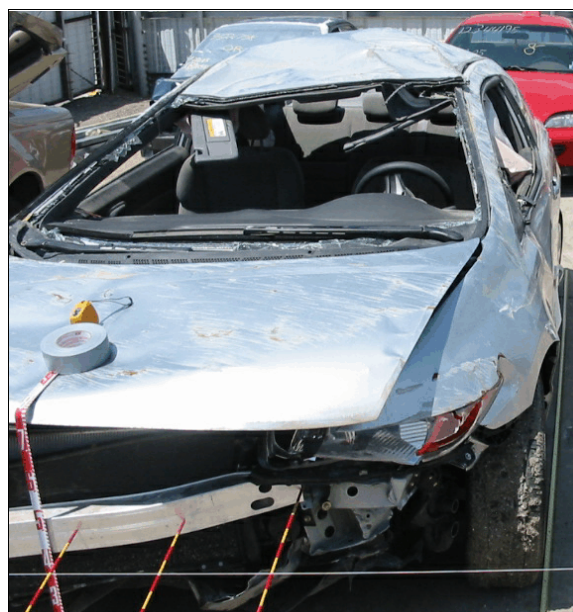
Figure 6: Rollover damage to hood, roof and upper left side
