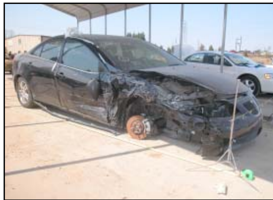
Figure 7. View of the front and right side damage to the G6.
