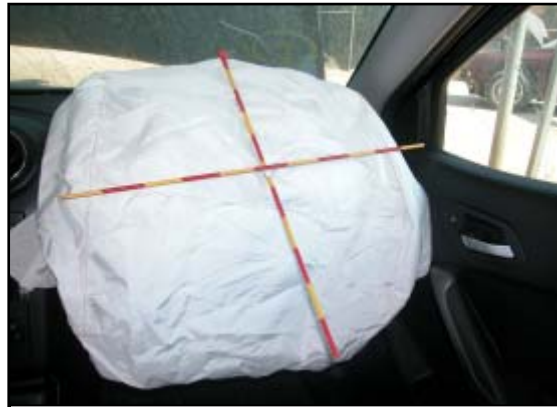
Figure 11. Deployed front right air bag.
