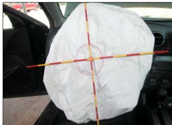
Figure 10. Deployed driver's frontal air bag.
