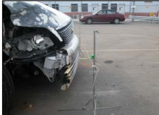
Figure 9. Lateral view of the residual crush to the bumper beam.
