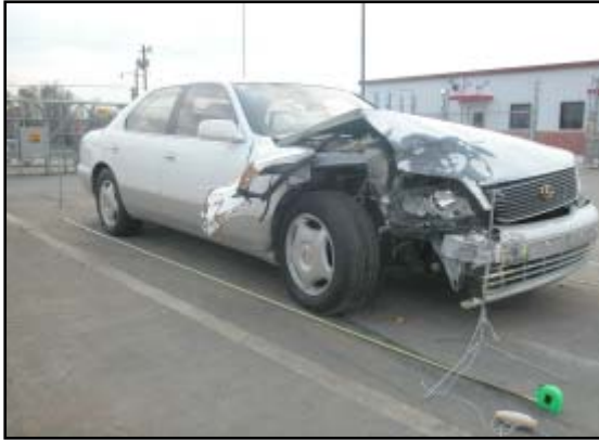
Figure 8. Front right view of the damage to the Lexus.
