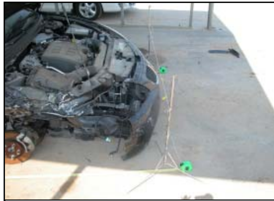
Figure 6. Upper support radiator crush to the G6.
