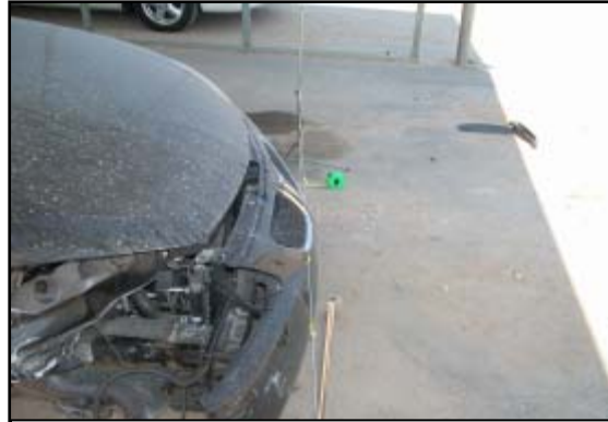
Figure 5. Lateral view of the front bumper of the Pontiac. No crush was noted at the bumper.
