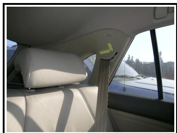
Figure 14. Scuff to left C pillar - possible occupant contact
