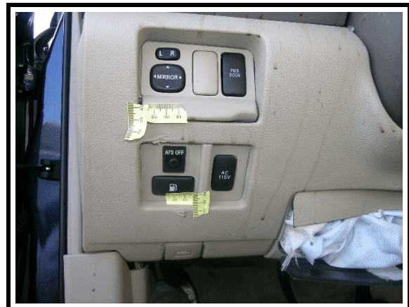
Figure 11. Possible occupant contact points - lower left instrument panel
