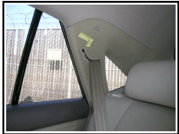
Figure 15. Scuff to right C pillar - possible occupant contact
