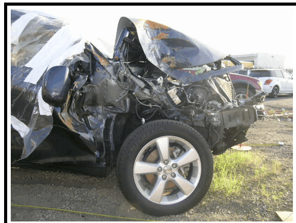
Figure 5. Damage to right front - 2005 Lexus RX330
