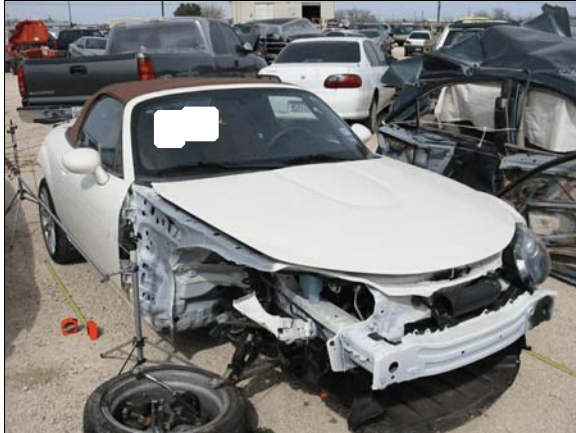
Figure 5: Right front overview of case vehicle, damaged right fender and front bumper had been removed and were not present at inspection facility
