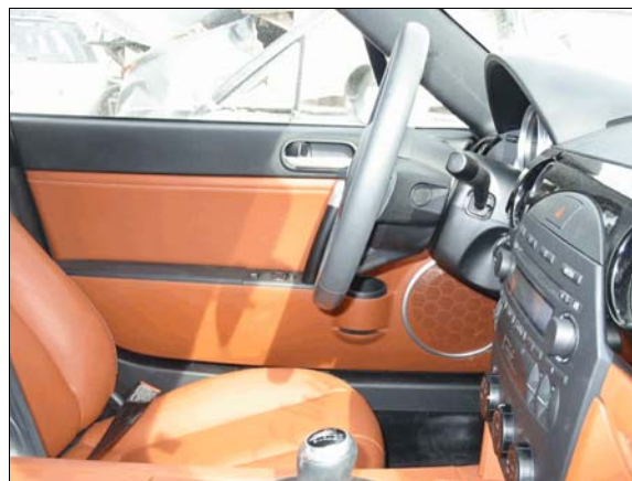
Figure 12: Right side view of case vehicle's steering wheel and steering column showing lack of deformation
