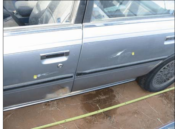
Figure 6: Damage to left front and left rear doors from impact with right quarter panel of case vehicle
