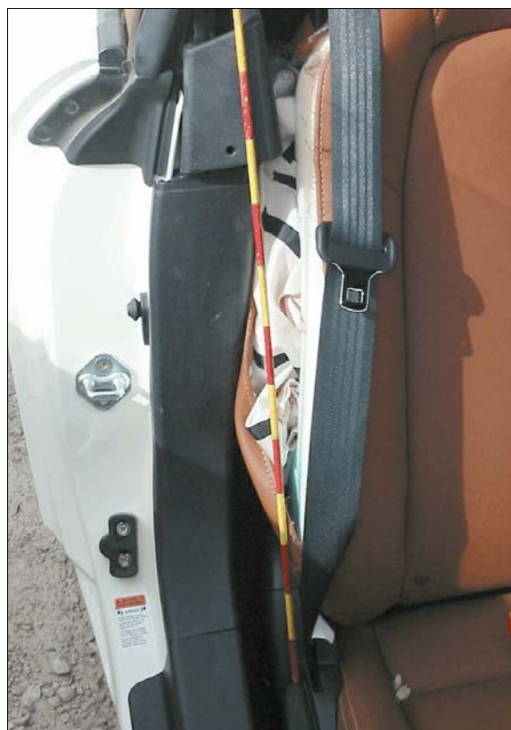
Figure 13: Case vehicle's front right passenger seat back-mounted side impact air bag located in right side of passenger seat back, each increment on rod is 5 cm (2 in)
