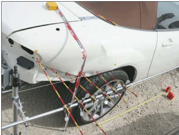
Figure 7: Damage to case vehicle's right quarter panel from side slap impact with the left side of the Toyota
