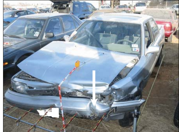
Figure 4: Overview of damage to front of Toyota from right fender impact with case vehicle, arrow shows location of stop sign impact
