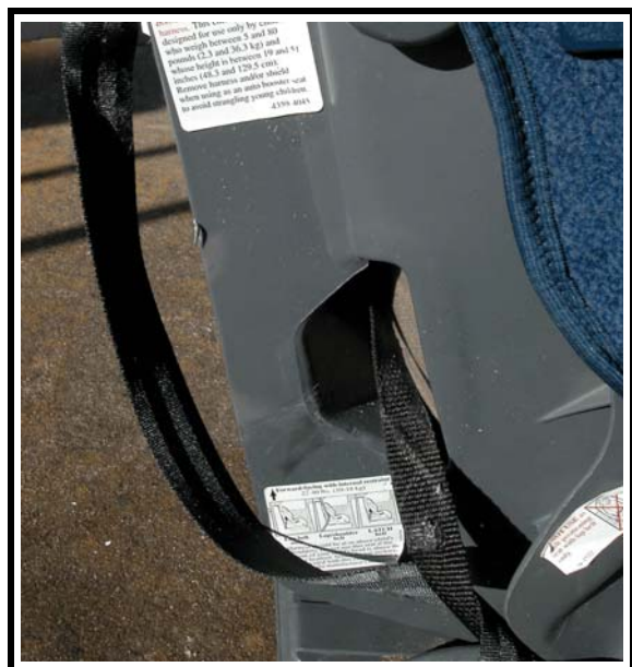
Figure 13. Loading marks to right side of child seat along belt path
