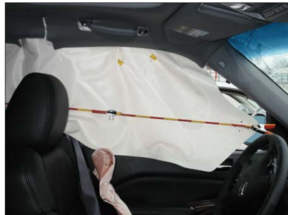
Figure 8: Case vehicle's driver side curtain air bag, each increment on rod is 5 cm (2 inches), yellow tape at top of bag shows two small black marks
