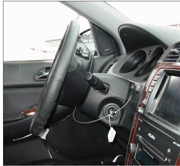
Figure 7: Right side view of case vehicle's steering wheel and steering column showing lack of deformation
