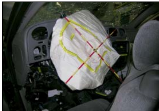
Figure 14. Deployed driver's frontal air bag.
