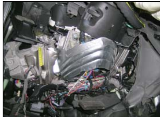
Figure 7. Compressed left bolster energy absorbing bracket and left shear capsule.
