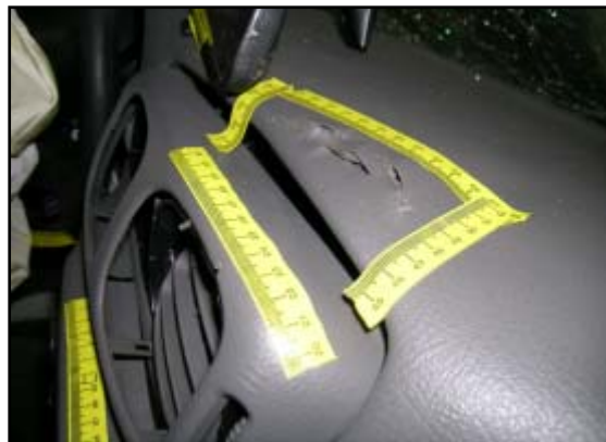
Figure 9. Upper center instrument panel contact from the rear left passenger.
