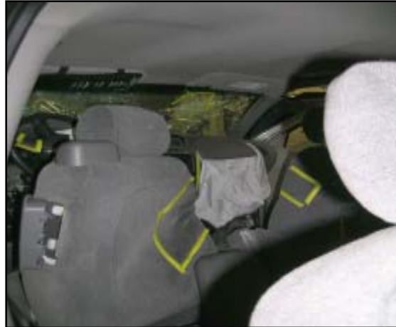
Figure 8. Rear left passenger's trajectory and contact points to the front seat backs.
