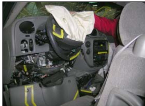
Figure 6. Driver's contact points to the steering wheel and knee bolster.
