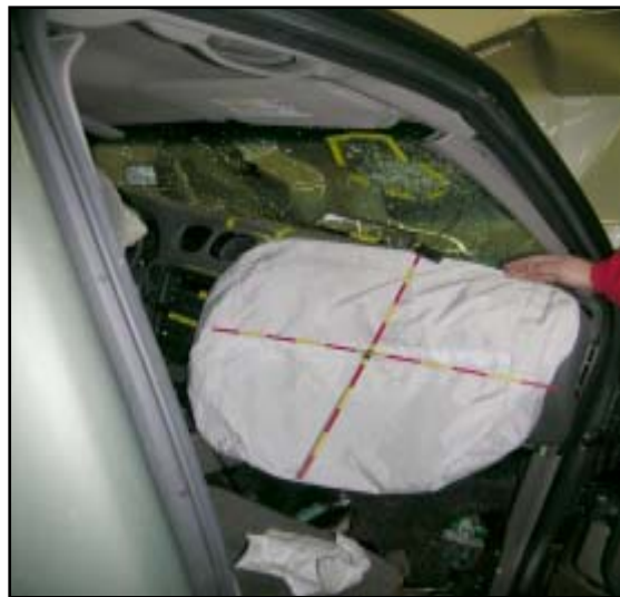
Figure 15. Deployed front right air bag.
