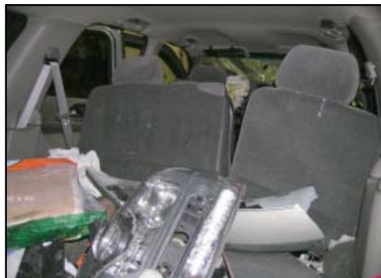
Figure 11. View of deformed rear seat backs from the rear cargo area.
