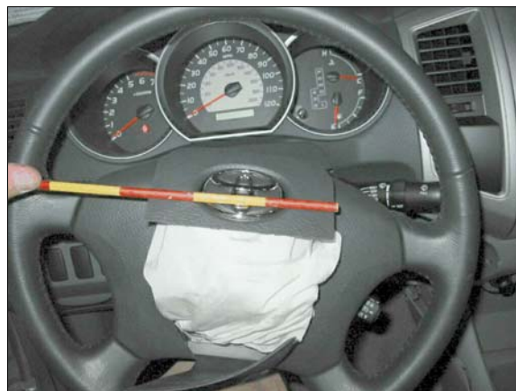
Figure 8: Case vehicle driver's air bag module cover flaps
