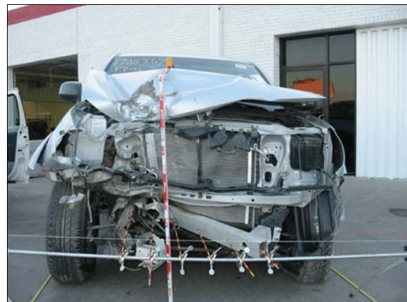
Figure 2: Overview of damage to front of case vehicle from impact with metal traffic signal poles, front bumper cover and grille have been removed, vertical scale in tenths of meters
