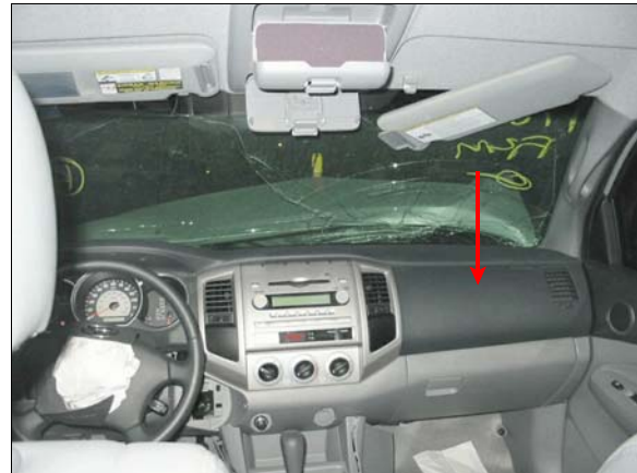
Figure 11: Overview of instrument panel, windshield and location of front right passenger's air bag, above glove box door
