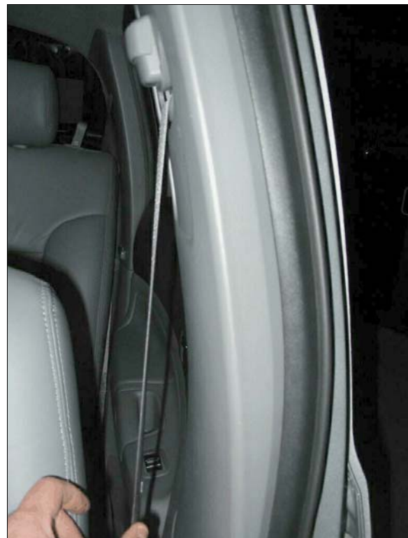
Figure 12: Case vehicle driver's safety belt jammed tightly in the retracted position indicating activation of the pretensioner
