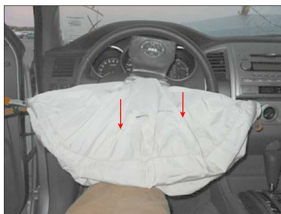
Figure 10: Arrows show locations of case vehicle's driver air bag vent ports
