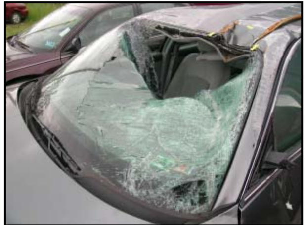
Figure 4: View of the roof deformation.
