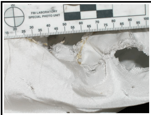
Figure 8. Burn/tear to upper right seam
