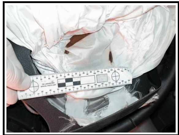
Figure 9. Melted portion of air bag at inflator
