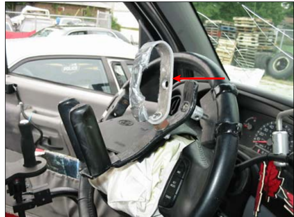
Figure 20: “Tri-Pin” type adaptive steering device attached to steering wheel, arrow shows palm grip modified with duct tape and apparently used as a hand grip
