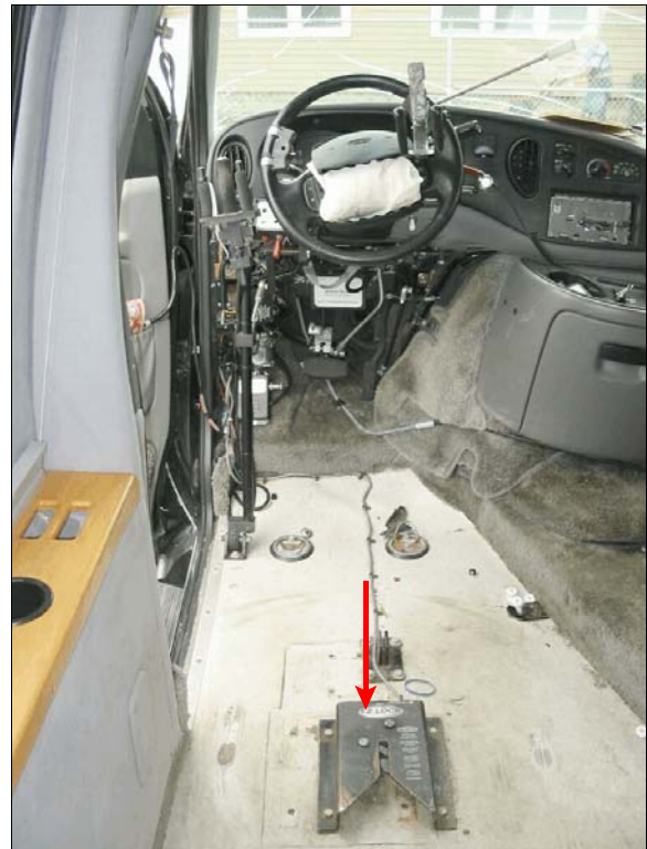
Figure 21: Overview of wheelchair anchor (arrow) and adaptive control equipment
