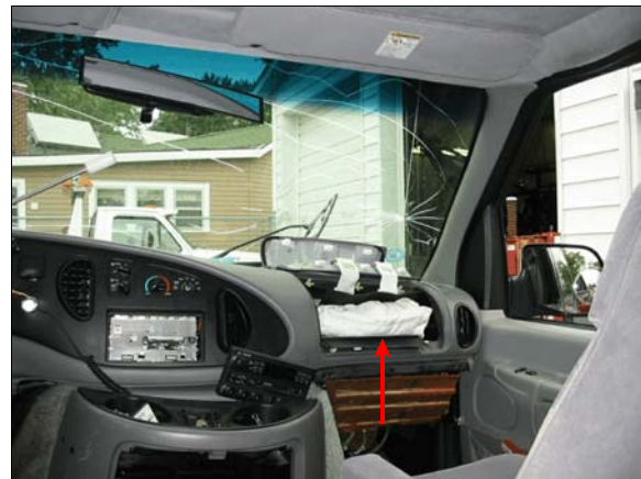
Figure 10: Overview of case vehicle’s center and right instrument panel, windshield and location of front right passenger air bag (arrow)
