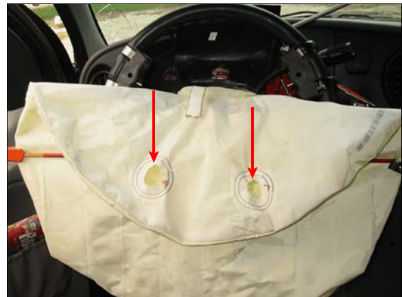
Figure 12: Case vehicle driver's air bag vent ports
