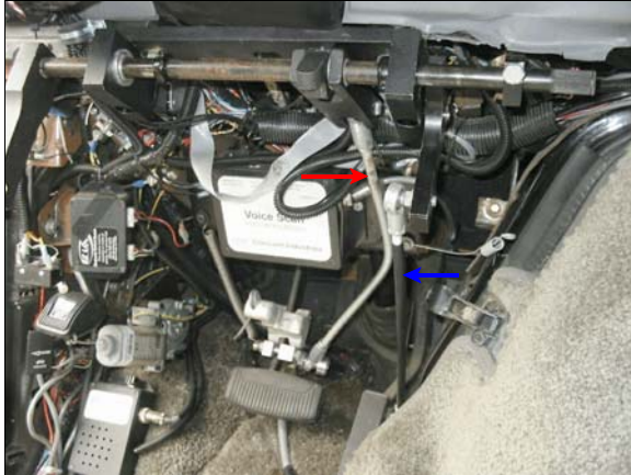
Figure 16: Red arrow shows brake actuator rod, blue arrow shows accelerator actuator rod, bend in brake actuator rod is not from occupant contact, it is bent to clear voice module
