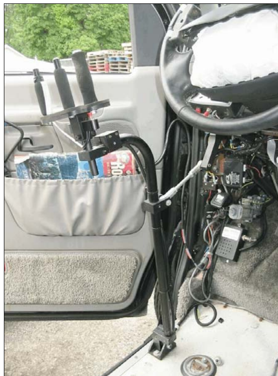
Figure 14: Overview of hand control, “joystick” and connector rod
