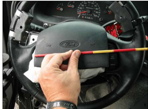
Figure 11: Case vehicle driver's air bag module cover flap
