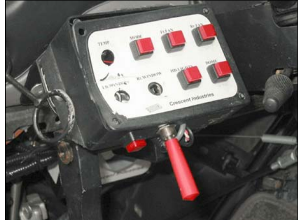
Figure 17: Damage to accessories control box mounted on left side of the steering wheel
