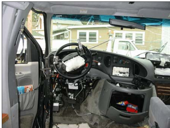
Figure 9: Overview of case vehicle’s steering wheel, instrument panel, windshield and adaptive control equipment
