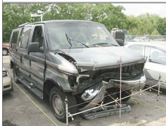
Figure 8: Front right overview of damage to case vehicle
