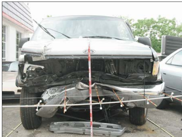
Figure 4: Damage to front of case vehicle from impact with the Honda, numbers on vertical scale are tenths of meter, each increment on rods is 5 cm (2 in)
