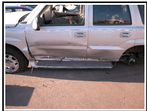
Figure 5. Left sill damage from impact with Honda
