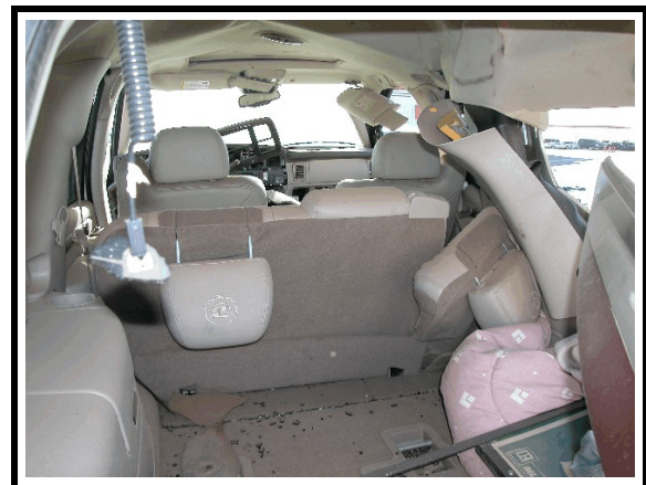
Figure 8. Overview of right side intrusion
