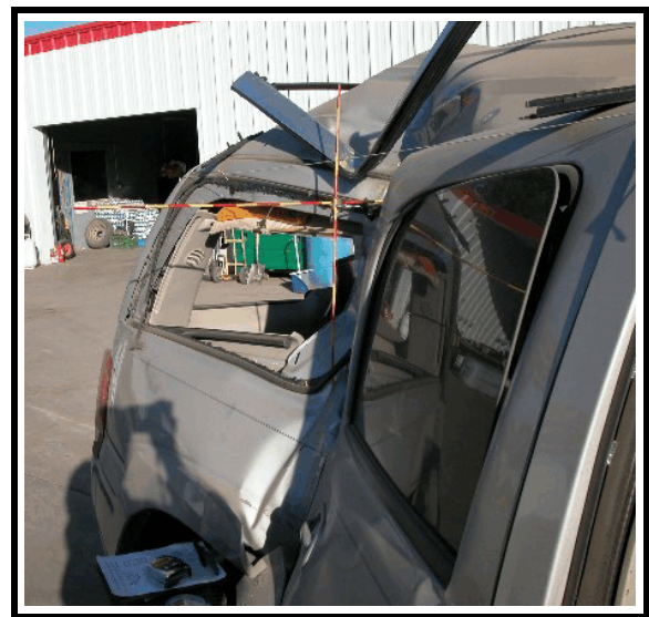
Figure 7. Lateral/vertical crush at the C pillar
