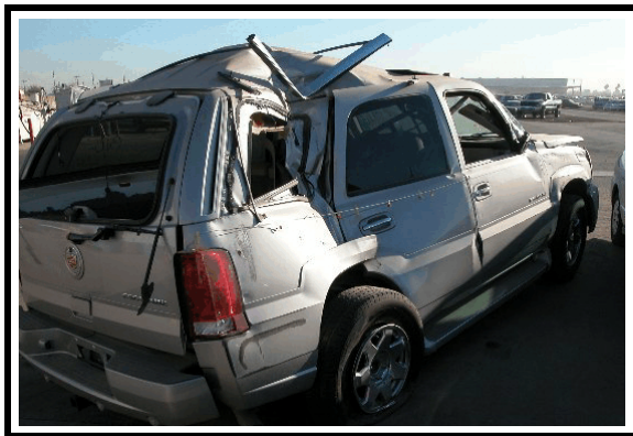
Figure 6. Right side pole and rollover damage
