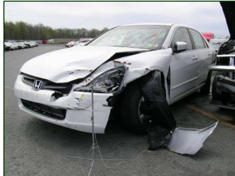
Figure 1. Frontal damage to the 2005 Honda Accord.
