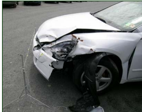
Figure 5. Lateral view identifying the extent of frontal crush and left side contact.
