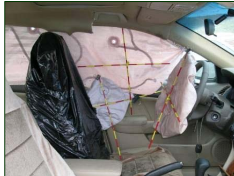
Figure 9. Deployed left side impact air bag and IC.
