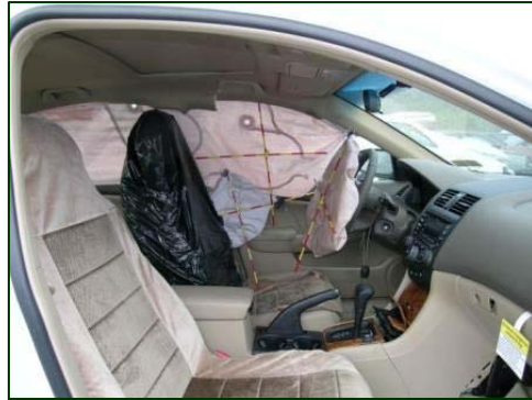
Figure 7. Lateral view of the driver's compartment and the deployed air bags.
