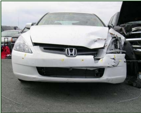
Figure 4. Frontal view of the front right corner damage to the Honda Accord.
