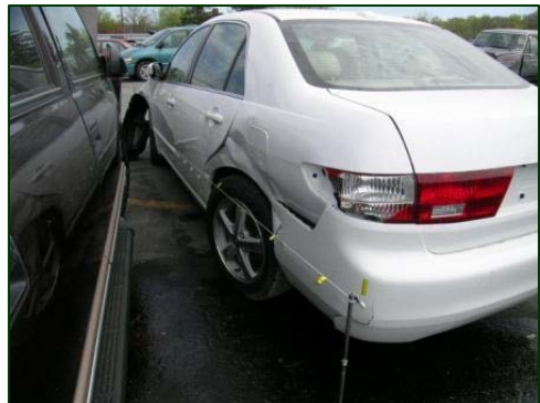
Figure 6. Left rear side damage to the Honda Accord.
