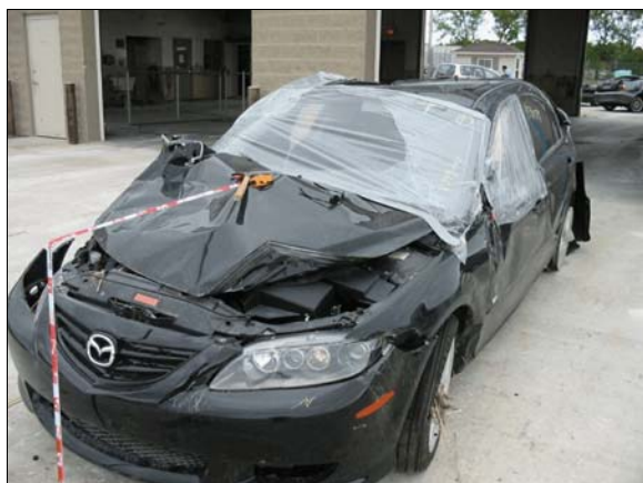
Figure 5: Overview of rollover damage to hood, roof and left side of case vehicle
