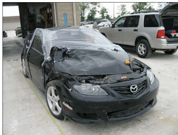
Figure 4: Overview of rollover damage to hood, roof and right side of case vehicle
