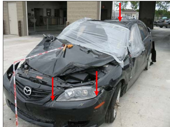
Figure 7: Overview of rollover damage to front and left side of case vehicle, arrows show scratches from fence impact
