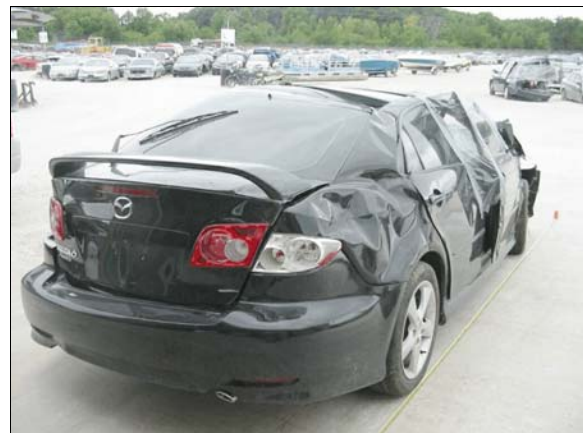
Figure 8: Overview of rollover damage to roof and right side
