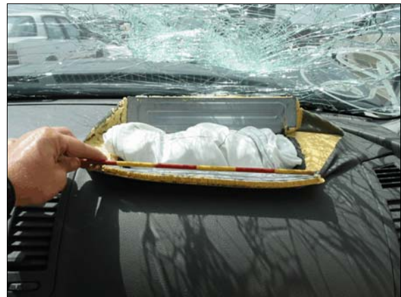
Figure 12: Case vehicle's front right passenger air bag module flaps, windshield is fractured due to contact by deploying front right passenger air bag
