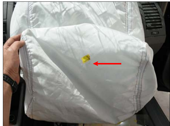
Figure 14: Overview of location of possible makeup scuff (arrow) at top central portion of front right air bag
