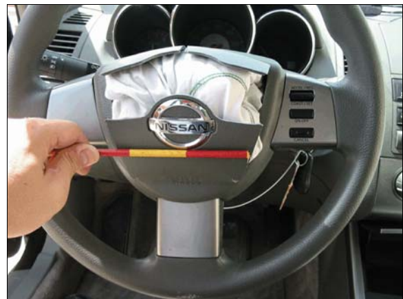
Figure 9: Case vehicle driver's air bag module cover flaps, each increment on rod is 5 cm (2 in)
