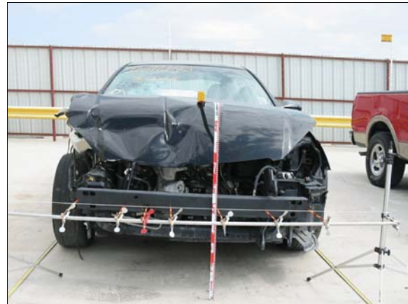
Figure 3: Overview of front damage to case vehicle due to impact with the back of the Honda, numbers on vertical scale are tenths of meter
