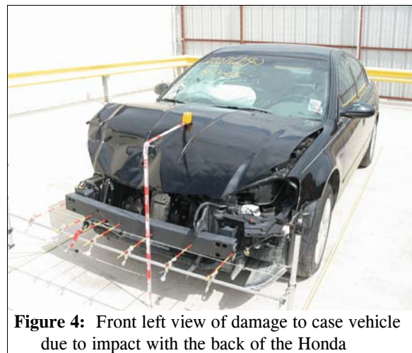
Figure 3: Overview of front damage to case vehicle due to impact with the back of the Honda, numbers on vertical scale are tenths of meter
