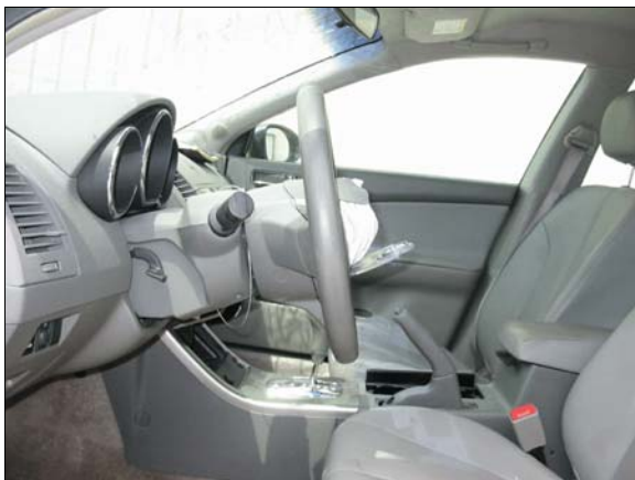
Figure 8: Left side view of case vehicle's steering wheel and column showing no deformation
