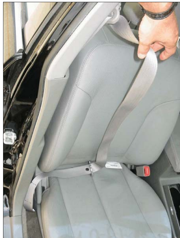
Figure 16: Front right passenger safety belt, retractor jammed with belt extended out of retractor, indicating activation of pretensioner while belt was in use
