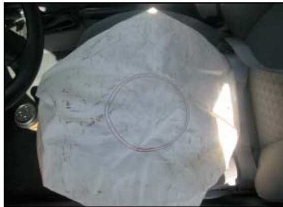
Figure 6. Deployed driver's frontal air bag.
