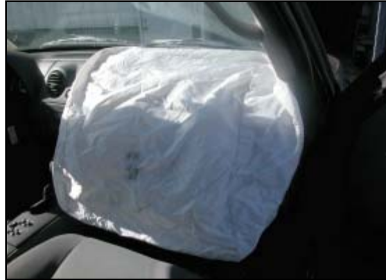
Figure 7. Deployed front right air bag.
