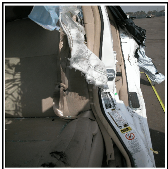
Figure 9. B pillar intrusion and trapped driver's seat belt
