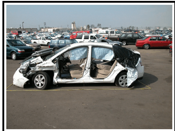
Figure 1. Left side damage - 2005 Toyota Prius
