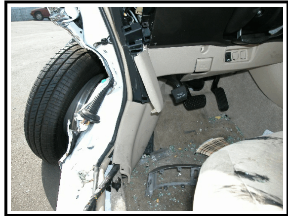
Figure 10. Intrusion into driver area
