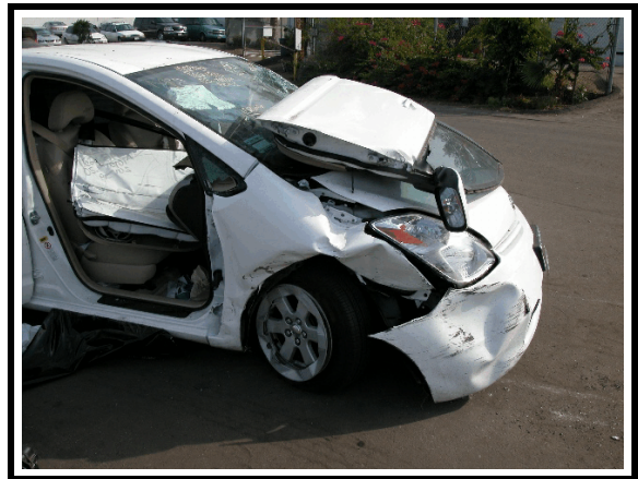
Figure 8. Damage to the right front of case vehicle
