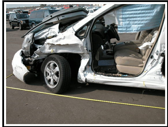
Figure 7. Damage to left front of case vehicle
