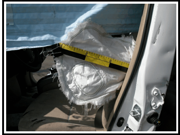
Figure 12. Driver's deployed side air bag
