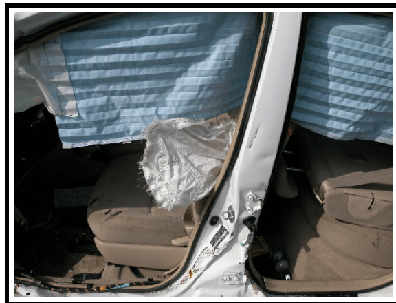
Figure 11. Deployed left side curtain and driver's seat back mounted air bag
