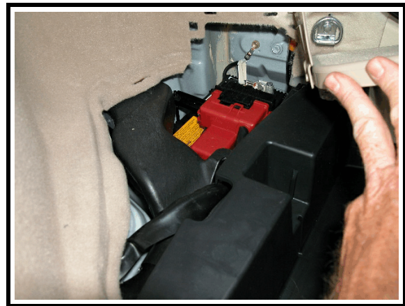
Figure 15. Battery service plug (power cutoff)
