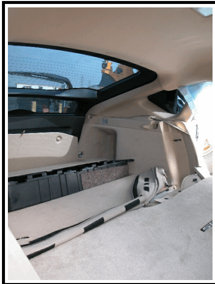
Figure 14. Traction battery located behind the second row seat back
