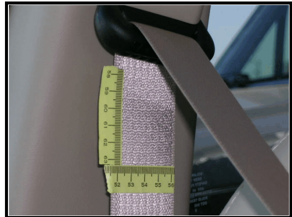
Figure 19. Evidence of loading to front right passenger's seat belt
