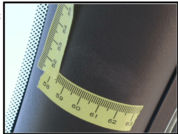
Figure 20. Close-up of occupant contact to right A pillar
