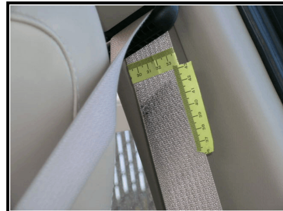
Figure 18. Evidence of loading to driver's seat belt
