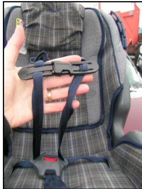
Figure 14: Close-up view the roped harness straps and chest clip.
