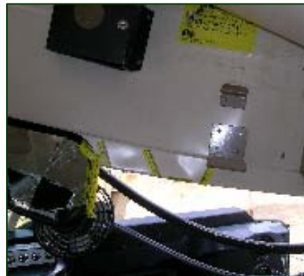
Figure 13. Student passenger head contact points to the mirror and header/bulkhead area.
