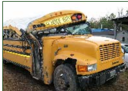
Figure 9. Impact area to the windshield header/A-pillar/bulkhead juncture.
