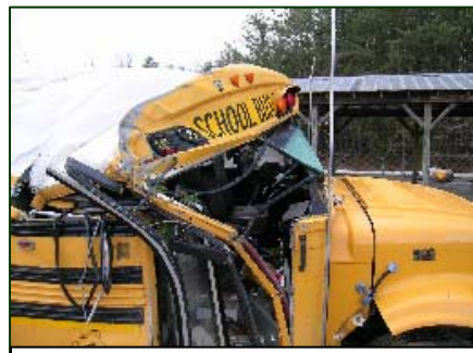
Figure 11. Extent of crush at the header area.
