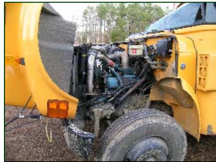
Figure 3. Engine compartment of the conventional chassis bus.
