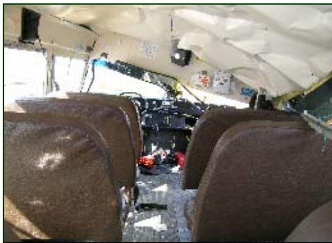
Figure 12. Intrusion/interior damage to the school bus.
