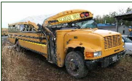
Figure 10. Primary impact damage to the header/A-pillar area.
