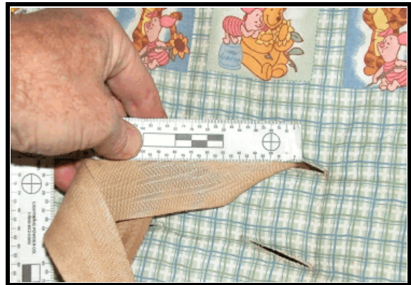
Figure 13. Scuff located on bottom of left side webbing
