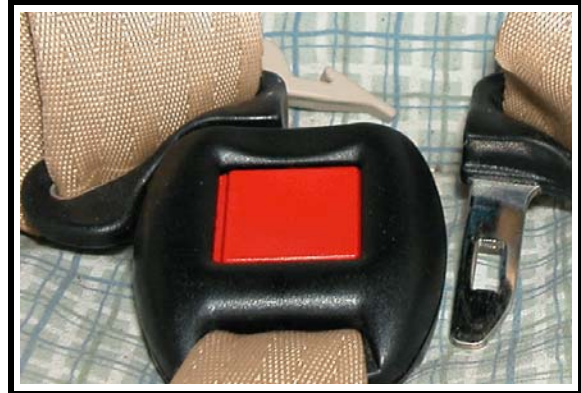
Figure 12. Child safety seat latch tongue
