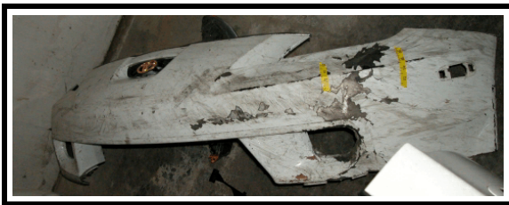
Figure 3. Initial contact area to front left bumper corner
