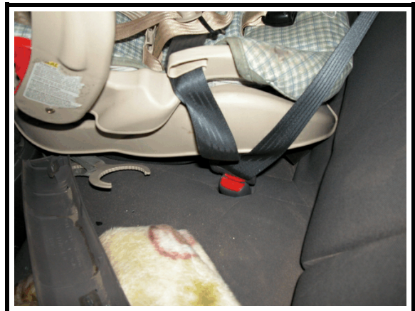
Figure 7. Rear right seat belt—used with infant seat
