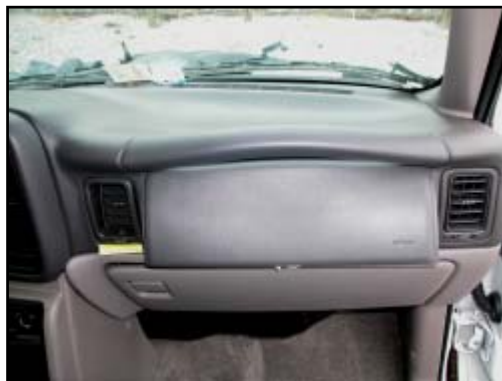
Figure 7. Close-up of right instrument panel damage from probable occupant contact
