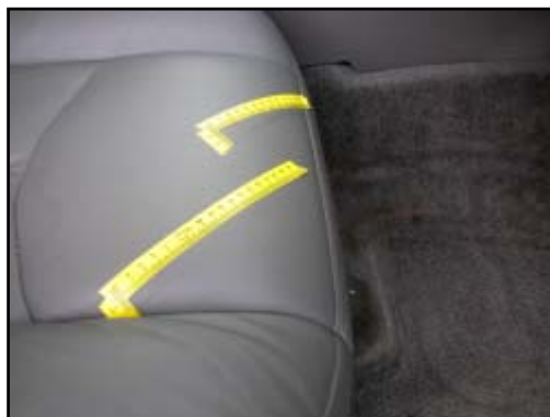
Figure 6. Scuff marks on front right seat
