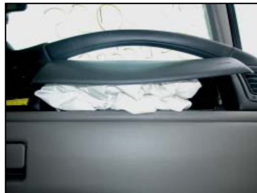
Figure 12. View from lower instrument panel showing damaged cover flap and lateral handle
