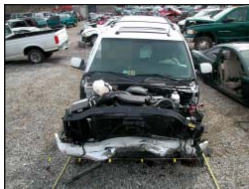
Figure 4. Frontal damage to the 2004 Chevrolet Suburban
