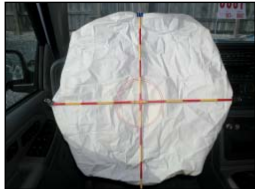
Figure 10. Deployed driver's air bag
