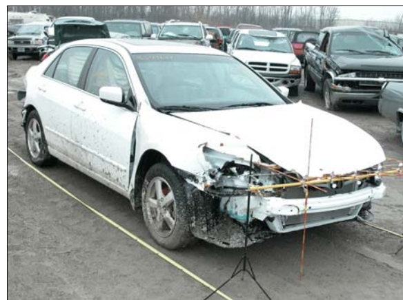
Figure 8: Overview of damage to case vehicle's front end and right quarter panel from guardrail impacts
