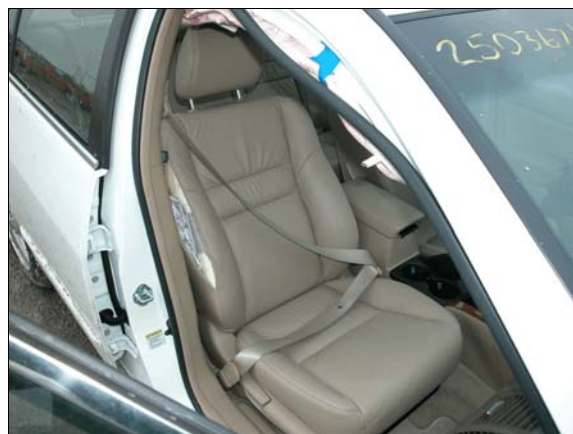
Figure 18: Front right passenger seat with safety belt buckled showing length of belt extended out of jammed retractor
