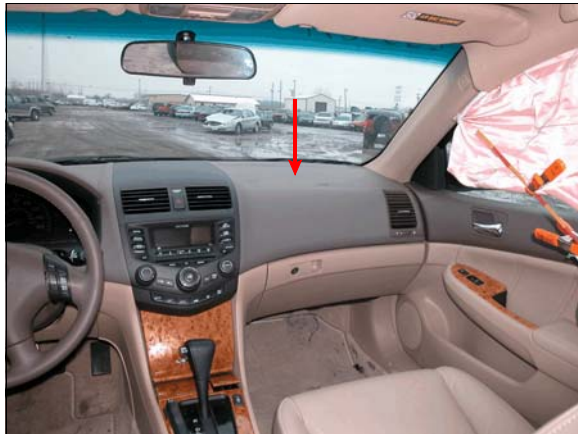
Figure 12: Overview of front right instrument panel, front right air bag located in top of instrument panel (arrow)
