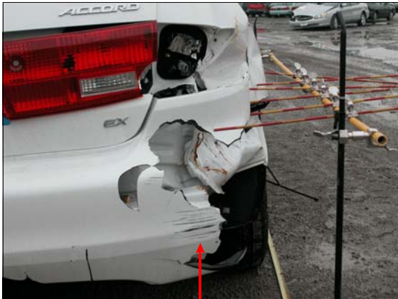
Figure 6: Damage to right corner of back bumper from impact with concrete bridge rail (arrow)
