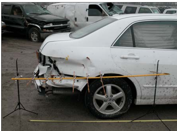
Figure 4: Damage to case vehicle’s right quarter panel from second impact with guardrail
