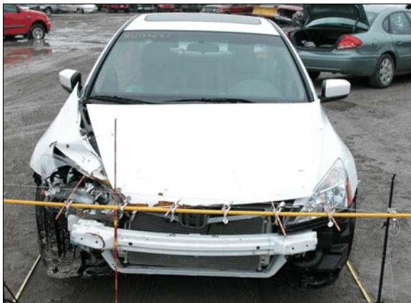
Figure 2: Damage to front of case vehicle from first impact with the guardrail
