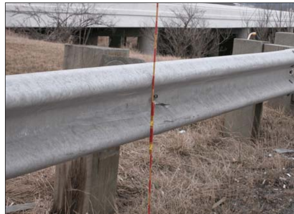
Figure 3: Location of case vehicle’s first impact with the guardrail, each stripe on rod is 5 cm (2 in)
