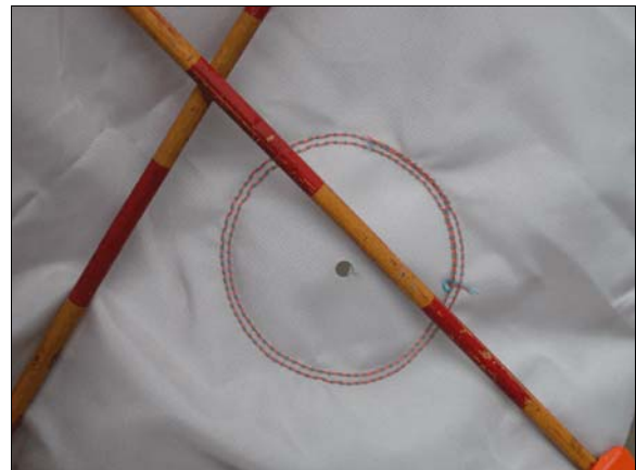
Figure 15: Circular stitch pattern in front right seat back-mounted side impact air bag
