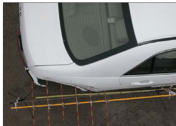
Figure 10: Top view of crush to case vehicle’s right quarter panel from second guardrail impact
