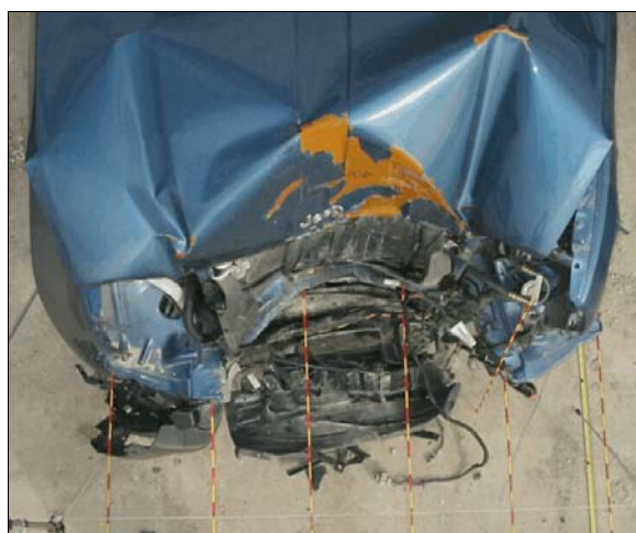
Figure 6: Top view of crush to front of case vehicle from impact with bridge support
