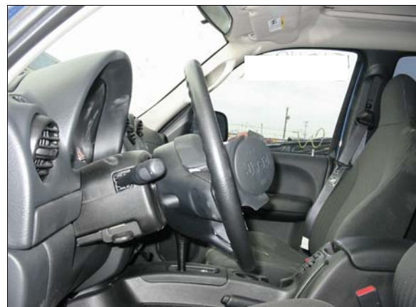
Figure 10: Case vehicle's steering column and steering wheel showing lack of deformation
