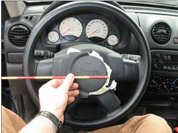
Figure 11: Case vehicle's driver air bag module flap
