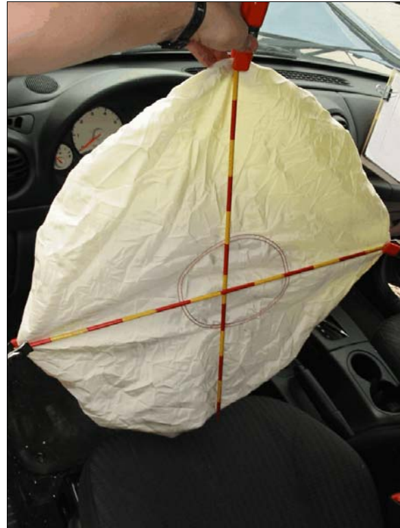
Figure 12: Case vehicle's driver air bag
