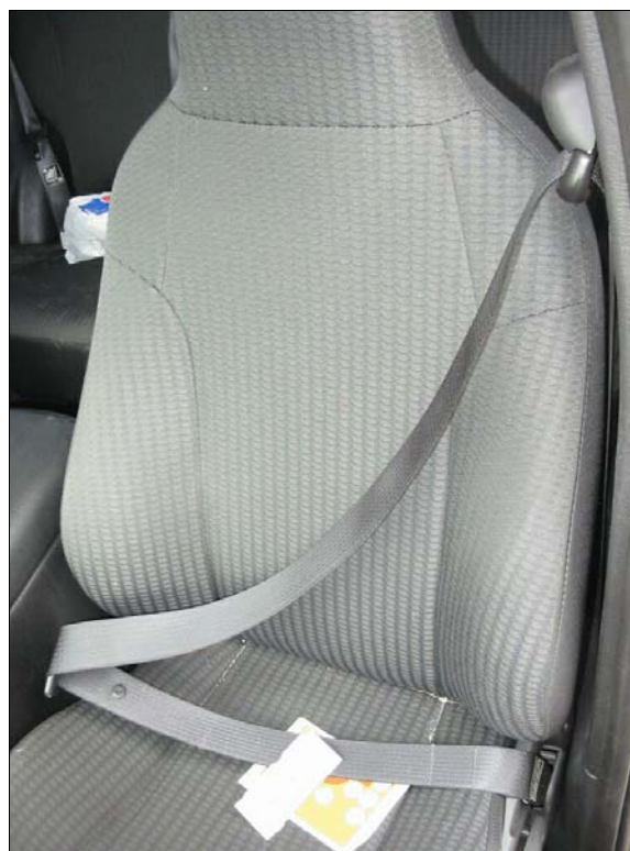
Figure 15: Case vehicle driver's safety belt in buckled position, retractor was jammed with length of belt spooled out of the retractor consistent with safety belt usage in the crash
