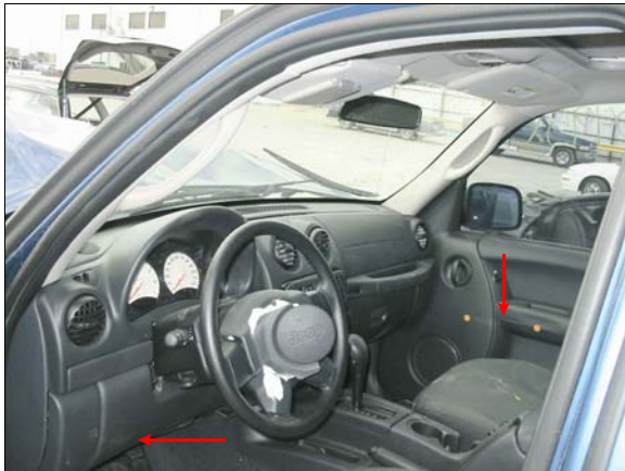
Figure 8: Overview of steering wheel and instrument panel, arrows show driver knee scuff on knee bolster and scuff on right front door
