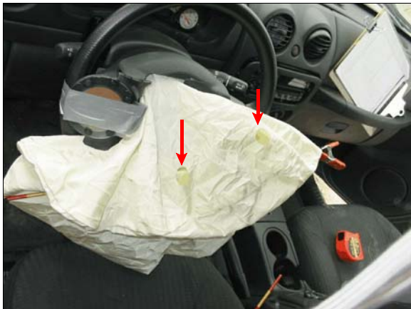
Figure 13: Top back portion of driver's air bag showing vent ports, indicated by arrows
