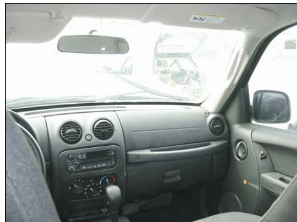
Figure 14: Front right passenger air bag located in middle of instrument panel above grab handle
