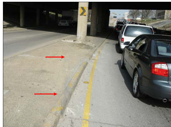
Figure 2: Case vehicle’s approach to impact with the concrete bridge support, arrow shows left front skid mark
