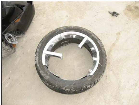
Figure 10: Damage to case vehicle's right front wheel from curb impact
