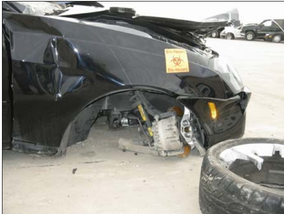
Figure 4: Damage to case vehicle's right front suspension and wheel due to curb impact
