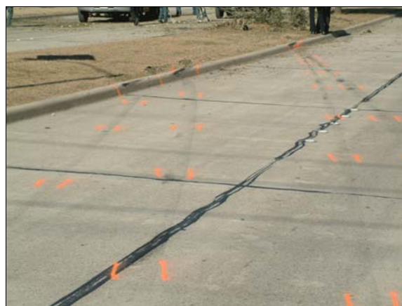
Figure 3: Police on-scene photo of case vehicle’s yaw marks and wheel impacts with curb; tire marks are, from left to right: left front, right front, left rear and right rear
