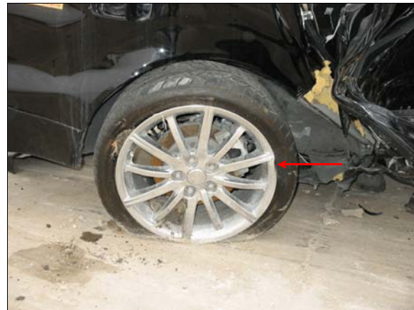
Figure 11: Dent in case vehicle's right rear rim (arrow) from curb impact, and dirt in bead and rim from furrowing into the ground adjacent to the curb
