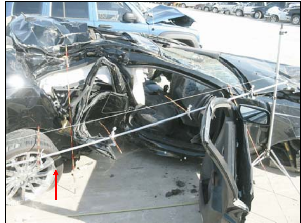
Figure 5: Damage to case vehicle's right side from tree impact [each increment on rod is 5 cm (2 in)], arrow shows dent in right rear rim from curb impact
