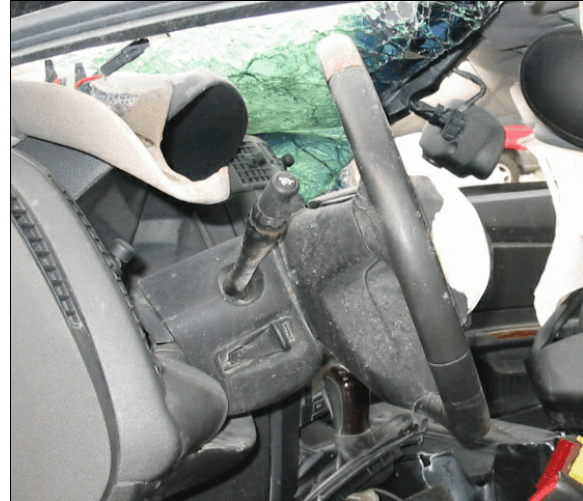
Figure 16: Left side view of steering column and steering wheel showing lack of deformation
