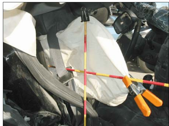
Figure 20: Right front, seat back-mounted, side impact air bag
