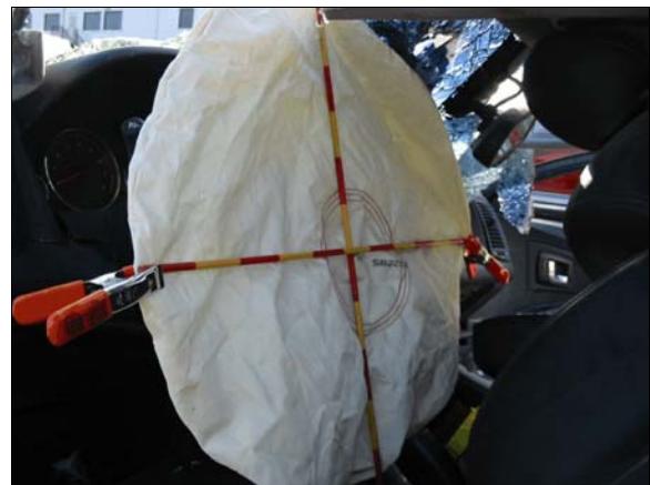
Figure 18: Driver's air bag, each increment on rods is 5 cm (2 in)
