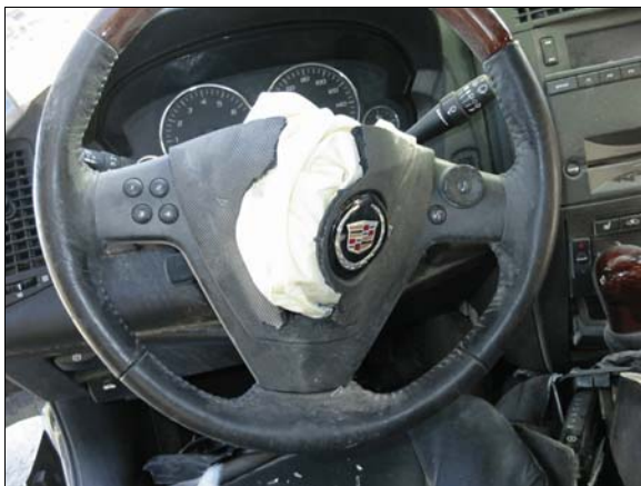
Figure 17: Case vehicle's driver air bag module flaps
