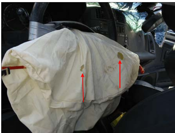
Figure 19: Driver's air bag vent ports (arrows)
