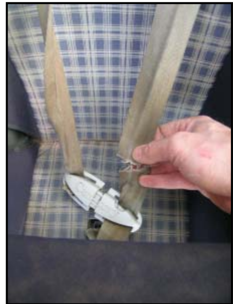
Figure 14: Close-up view of the harness straps and retainer clip.
