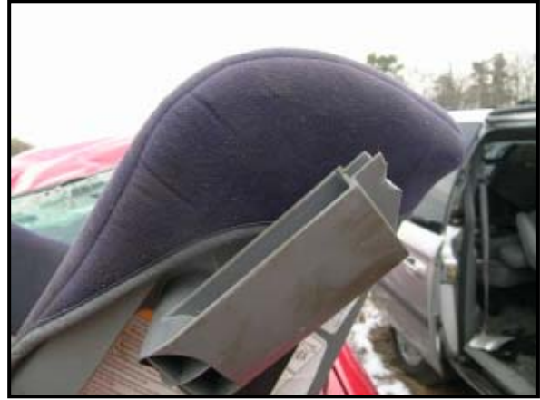
Figure 12: Fractured tray shield support.
