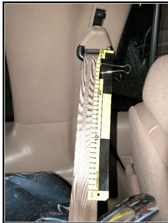
Figure 6. Loading/scuff marks to second row, left side safety belt
