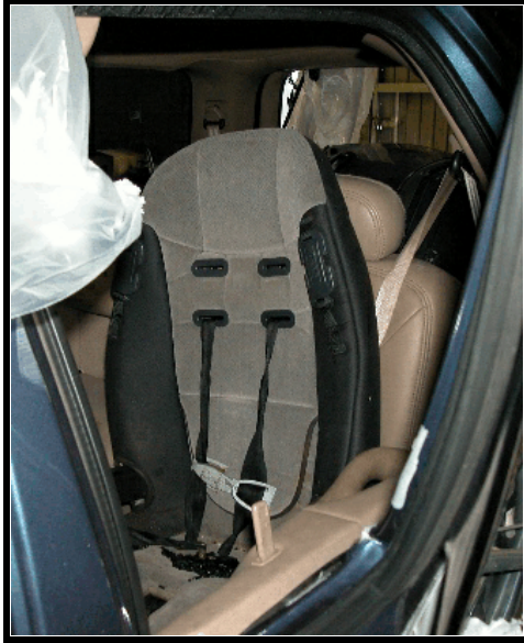
Figure 10. Century child seat. Scuff to seat back from shoulder belt.
