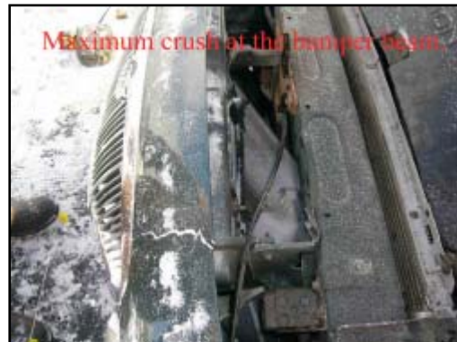
Figure 6. Close up of the impact damage.
