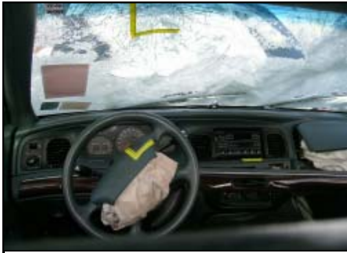
Figure 8. Driver's windshield contact.
