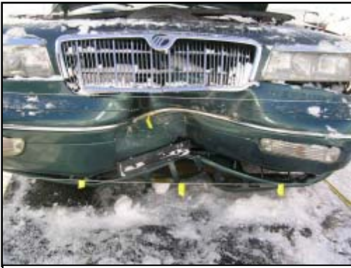
Figure 5. Resultant damage from the pole impact.
