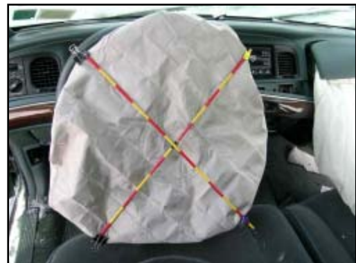
Figure 10. Deployed driver's air bag.
