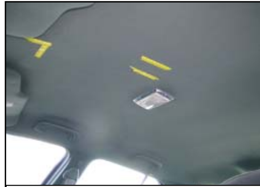
Figure 9. Headliner contact points.
