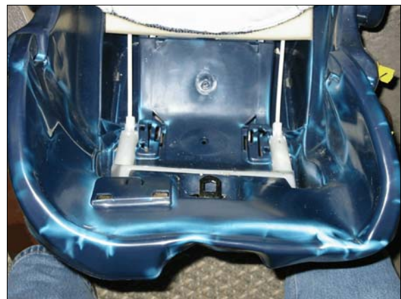
Figure 14: Deformation to bottom section of the infant seat
