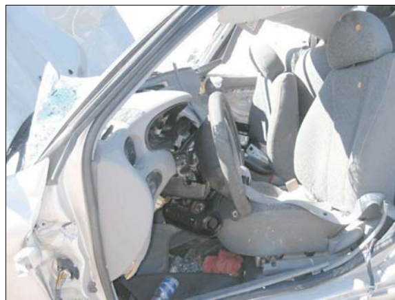
Figure 18: Intrusion of case vehicle's instrument panel and displacement of steering wheel entrapped driver legs
