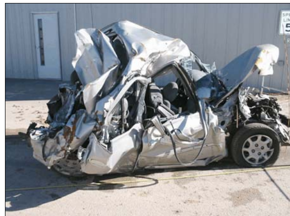
Figure 4: Right side overview of damage to back and front of the case vehicle
