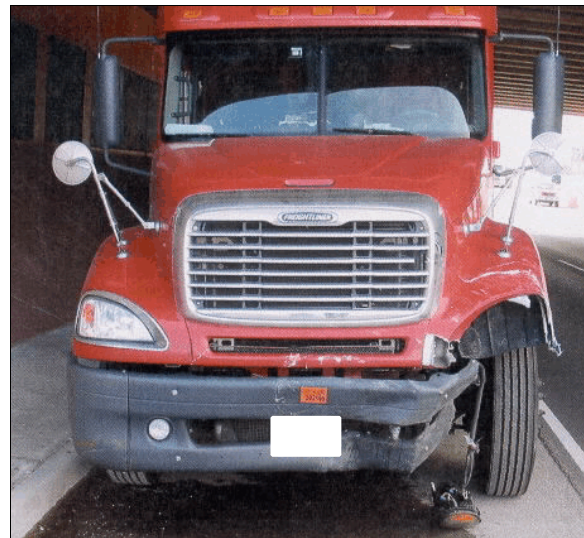
Figure 3: Overview of damage to front of Freightliner from impact with back of case vehicle
