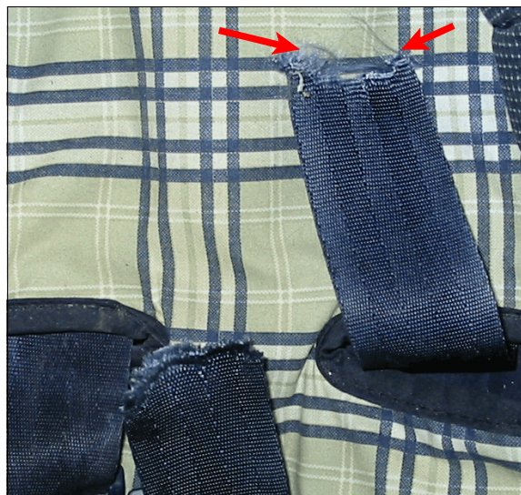
Figure 16: Separated ends of the infant seat’s left harness strap, arrow shows ragged strands of webbing fibers on edges of strap
