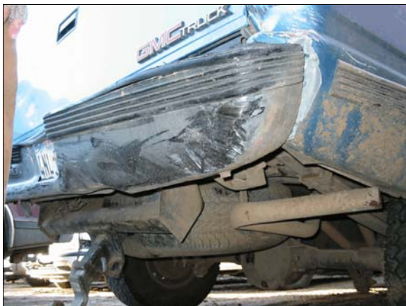
Figure 7: Damage to GMC back right corner due to impact with case vehicle's right front side
