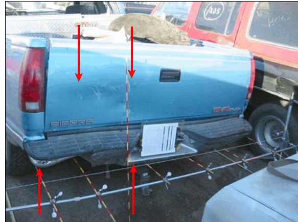
Figure 6: Direct damage to back left of GMC (arrows) due to impact with front right of case vehicle
