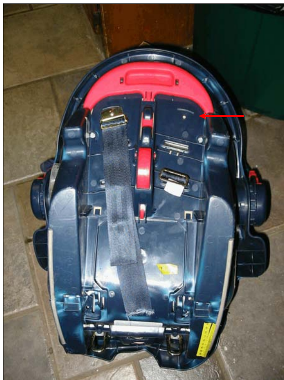
Figure 13: Back of infant seat showing stress marks on bottom of seat, harness strap and missing harness anchor (arrow)
