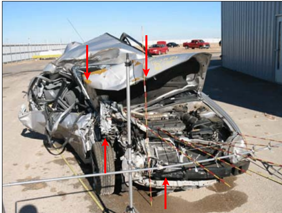
Figure 5: Direct damage to front right of case vehicle (arrows) due to impact with the back left of the GMC, each stripe on rods is 5 cm (2 in)
