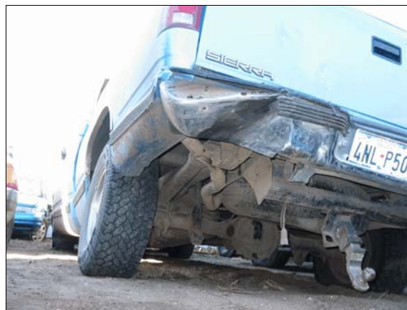
Figure 15: Underride damage due to impact by case vehicle’s front right
