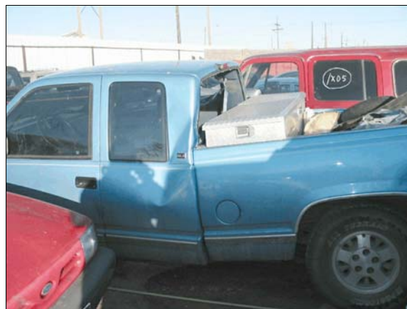
Figure 16: Induced damage to back of cab and bed
