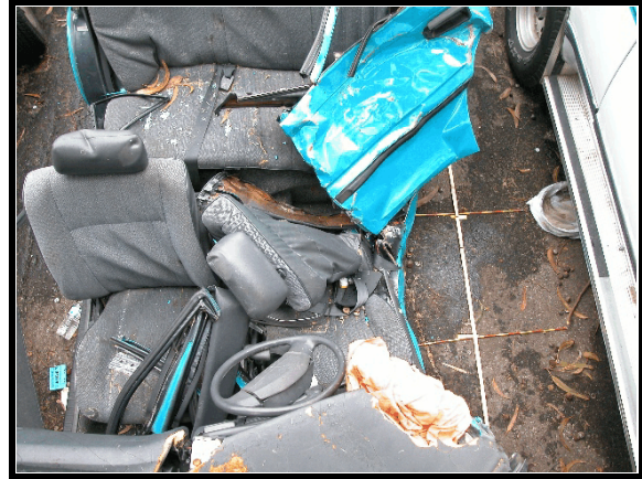
Figure 8. Overview of left side intrusion damage
