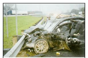
Figure 3: Left side of case vehicle at final rest; note, slight bending of guardrail
