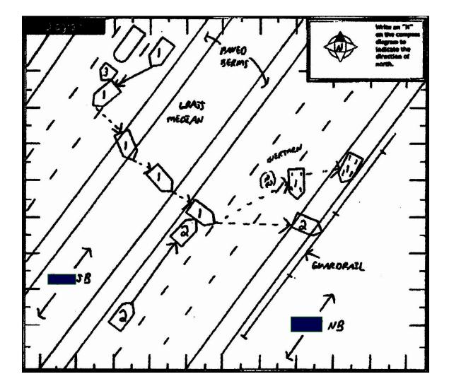
Copied from the police crash report. The case vehicle is V2 in this drawing. V1 is the Jeep and V3 is the Volvo tractor-trailer rig. The Mercury Sable (third other vehicle) is not depicted in this drawing.
