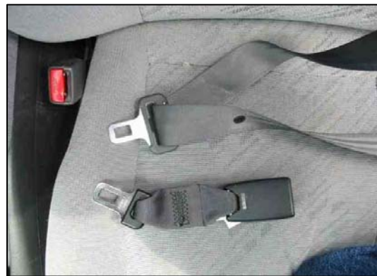
Figure 8 - Disengaged safety belt extender.
