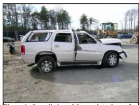
Figure 4. Overall view of the crush to the roof side rail.
