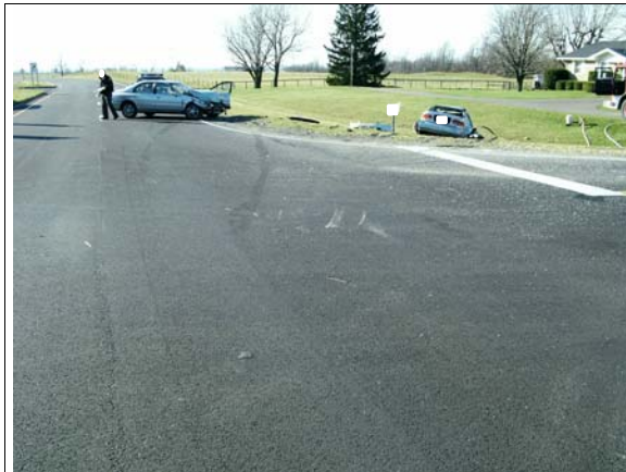
Figure 3: On-scene photo of impact gouges, post impact tire marks and final rest positions of case vehicle and V2
