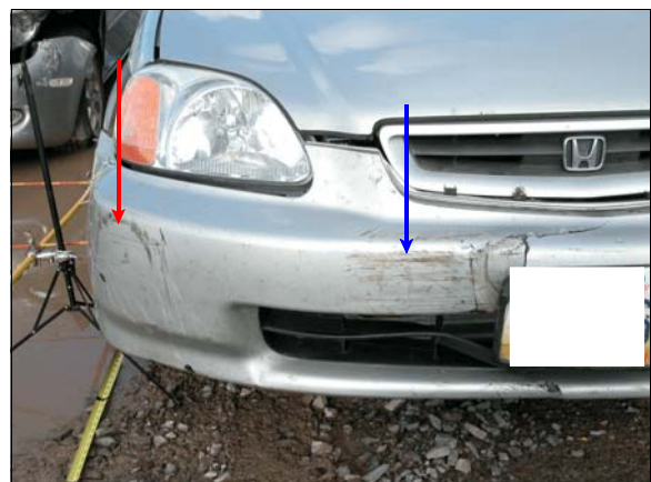
Figure 7: Damage to V2's front bumper from county road sign impact (blue arrow) and secondary impact to right fender and bumper corner of case vehicle (red arrow)
