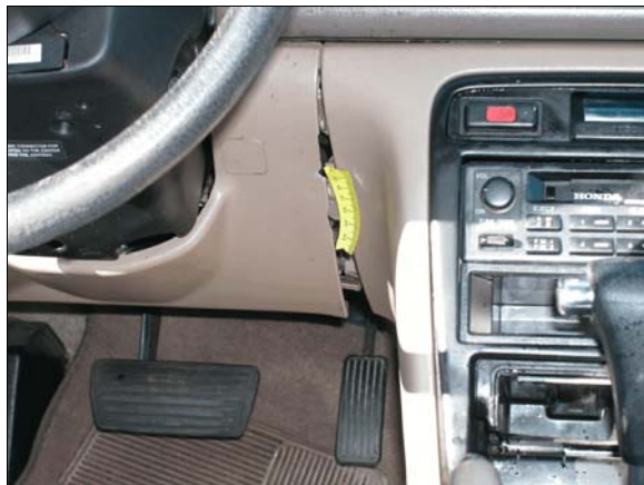
Figure 11: Damage to case vehicle's right knee bolster due to impact by driver's right knee
