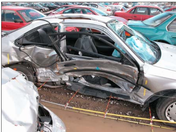
Figure 5: Damage to right side of V2, yellow tape below door handle is center of direct damage
