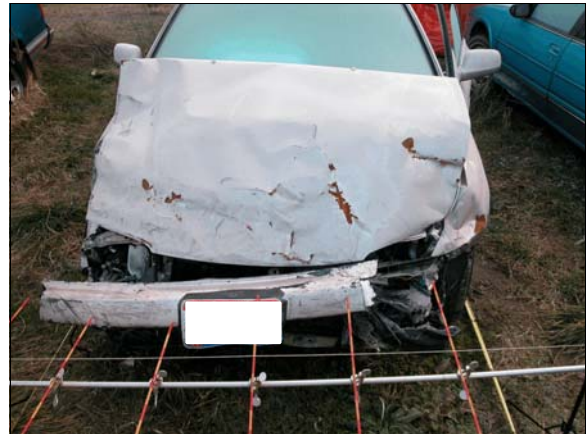
Figure 4: Damage to front of case vehicle due to impact with right side of V2, bumper placed back on vehicle for measurement
