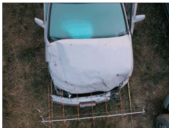
Figure 9: Top view of case vehicle's hood level crush
