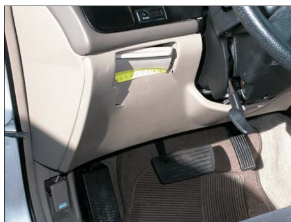
Figure 10: Damage to case vehicle’s left knee bolster from impact by driver’s left knee
