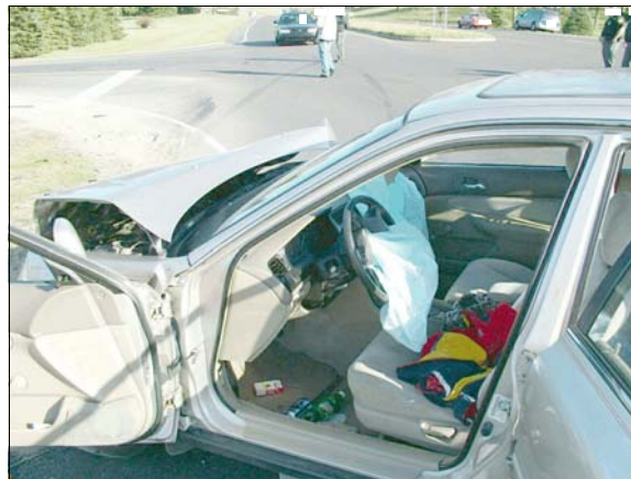
Figure 12: On-scene photo of case vehicle's driver air bag, steering wheel and steering column
