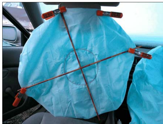
Figure 13: Case vehicle's driver air bag, steering wheel is rotated CW about 170 degrees
