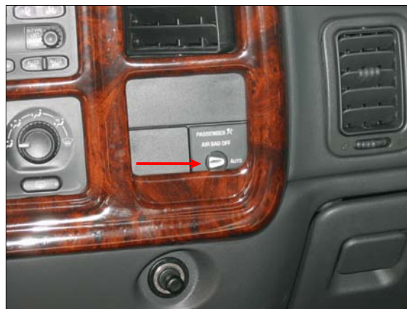
Figure 13: Front right passenger air bag suppression switch set to "AUTO"
