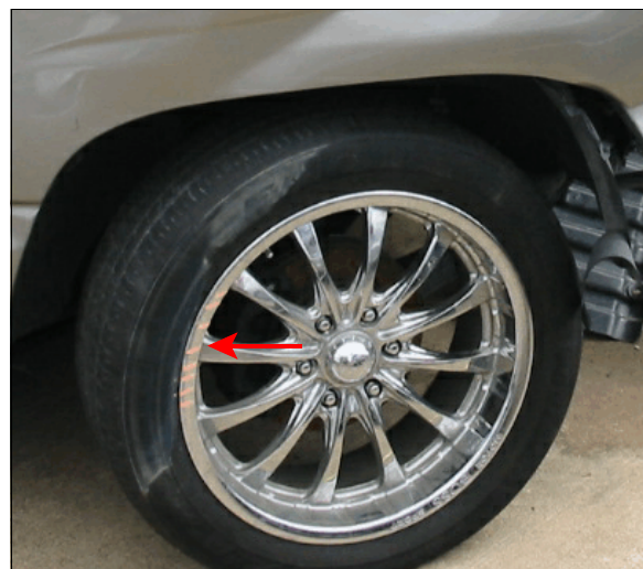
Figure 4: Damage to case vehicle's right front wheel rim
