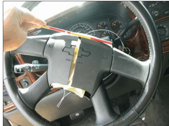
Figure 11: Case vehicle’s driver air bag module flaps
