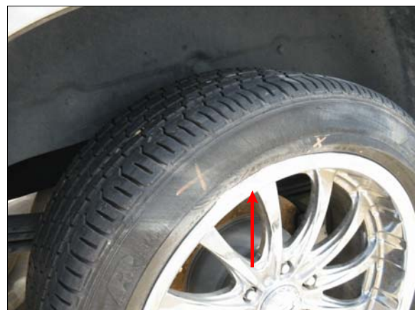
Figure 5: Damage to case vehicle's right rear wheel rim and tire
