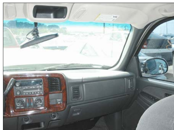
Figure 12: Overview of front right air bag location in middle of instrument panel above glove box
